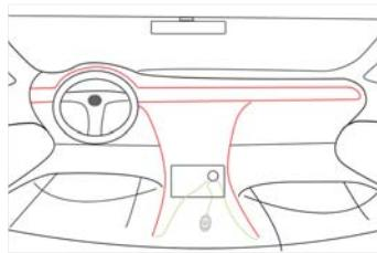
②: Turn off the power, Confirm the installation position, and optical fiber along these gaps.
