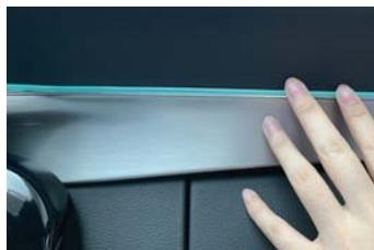
④: Press the optical fiber into the gap.
