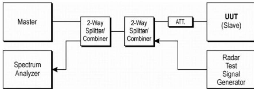
Figure 3-1. Conducted Test Setup for DFS
