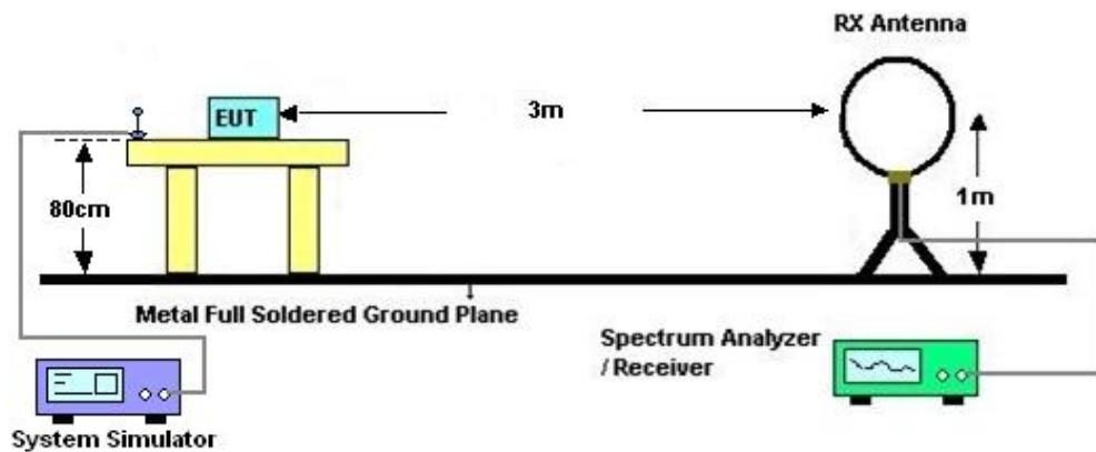
For radiated test from 30MHz to 1GHz
