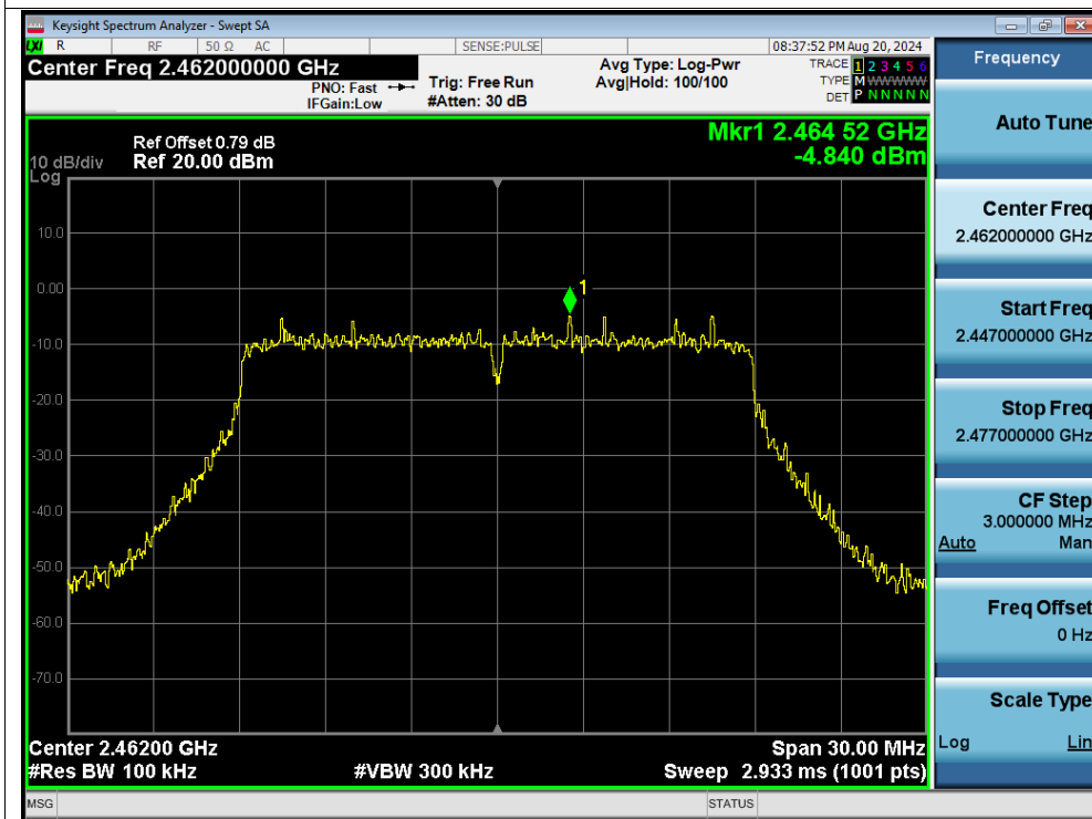
Band Edge NVNT n20 2462MHz Ant1 Emission
