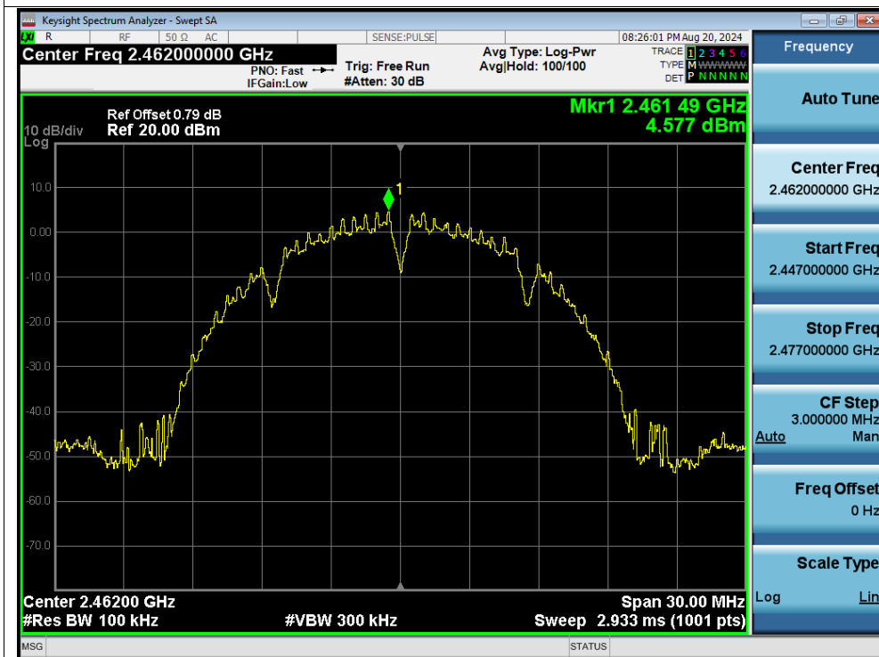
Tx. Spurious NVNT b 2462MHz Ant1 Emission
