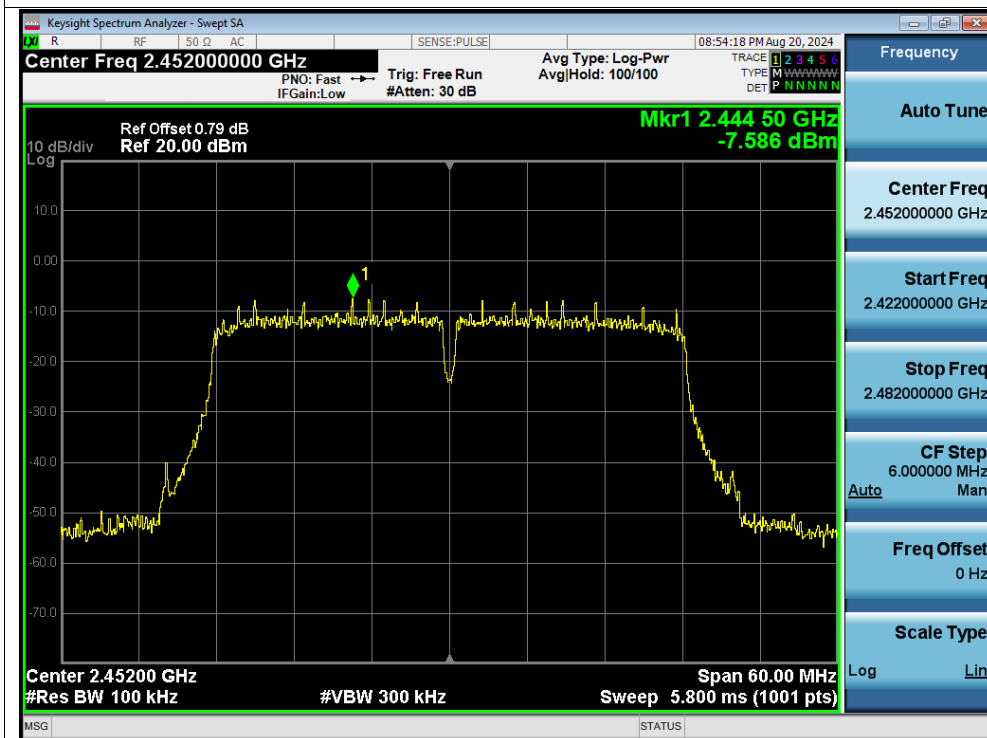
Band Edge NVNT n40 2452MHz Ant1 Emission
