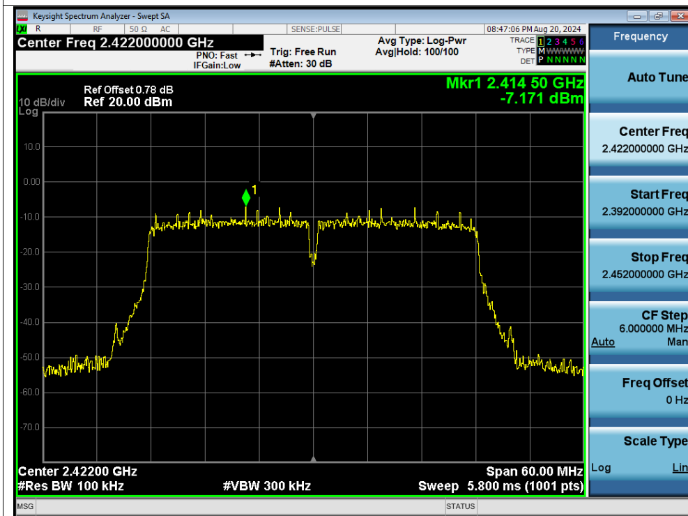
Band Edge NVNT n40 2422MHz Ant1 Emission
