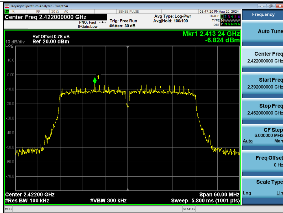
Tx. Spurious NVNT n40 2422MHz Ant1 Emission
