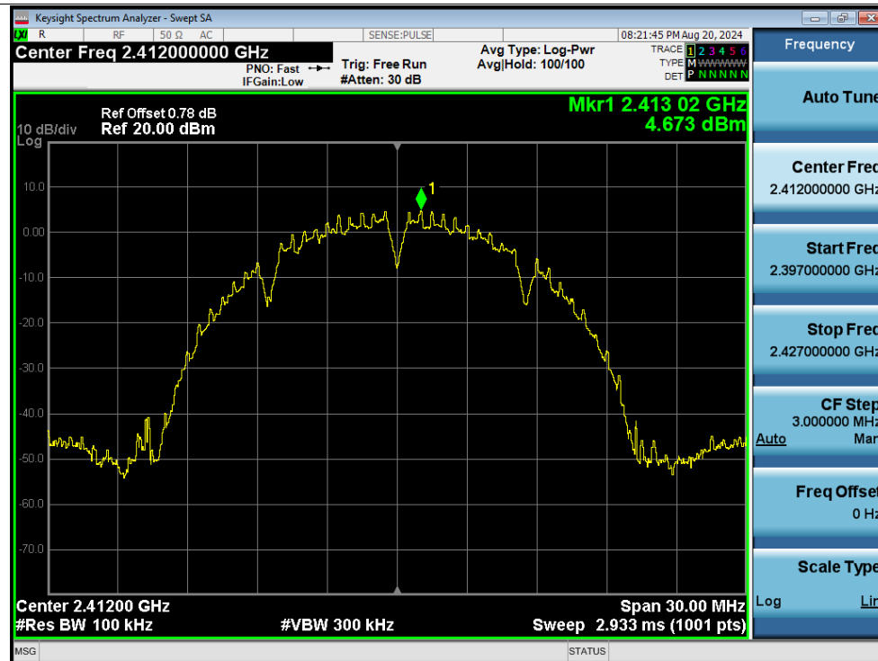
Tx. Spurious NVNT b 2412MHz Ant1 Emission
