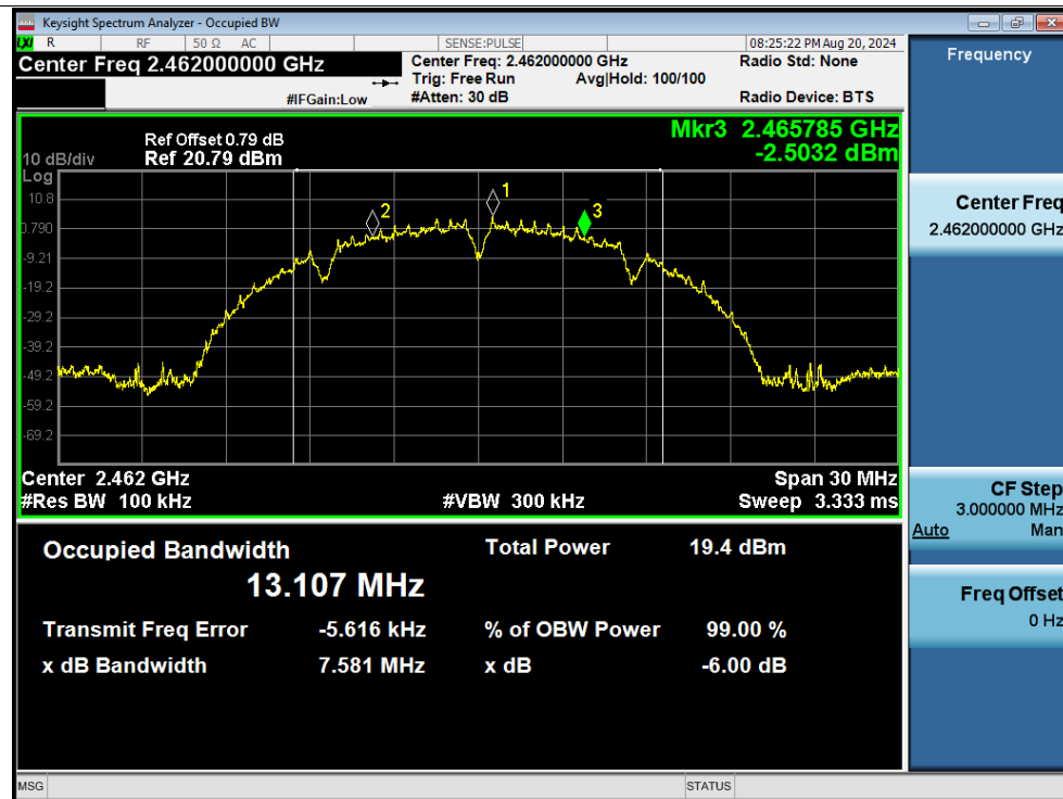
-6dB Bandwidth NVNT g 2412MHz Ant1
