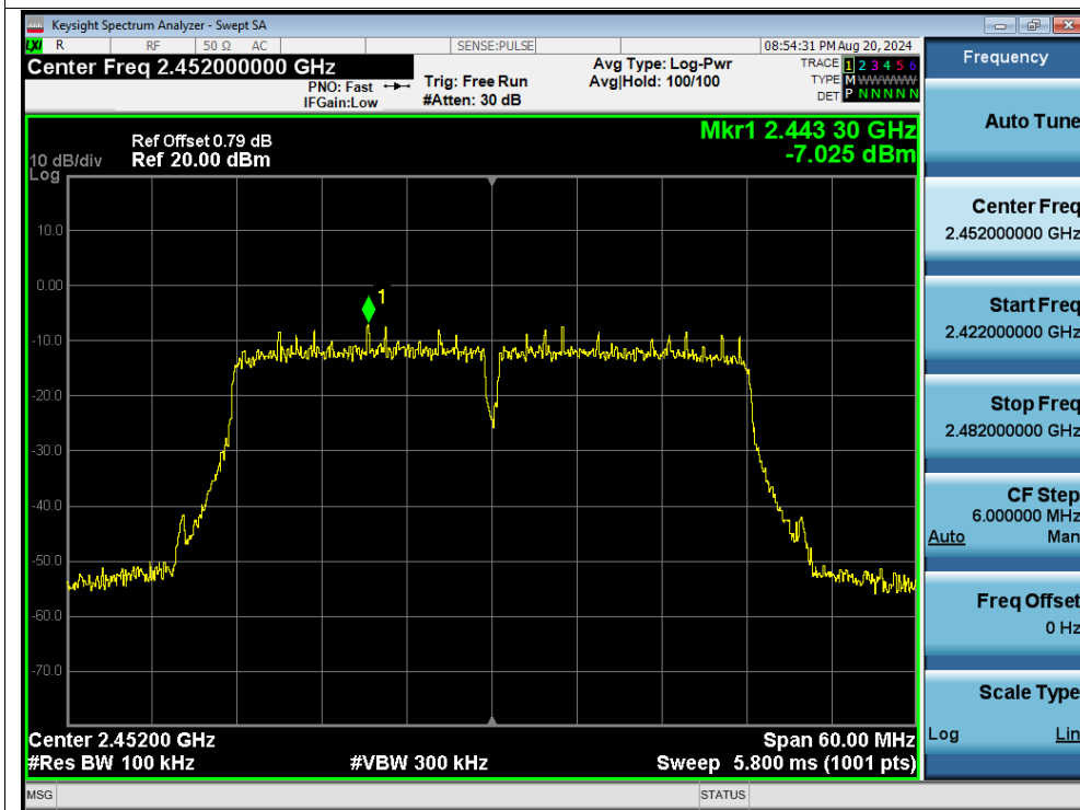
Tx. Spurious NVNT n40 2452MHz Ant1 Emission
