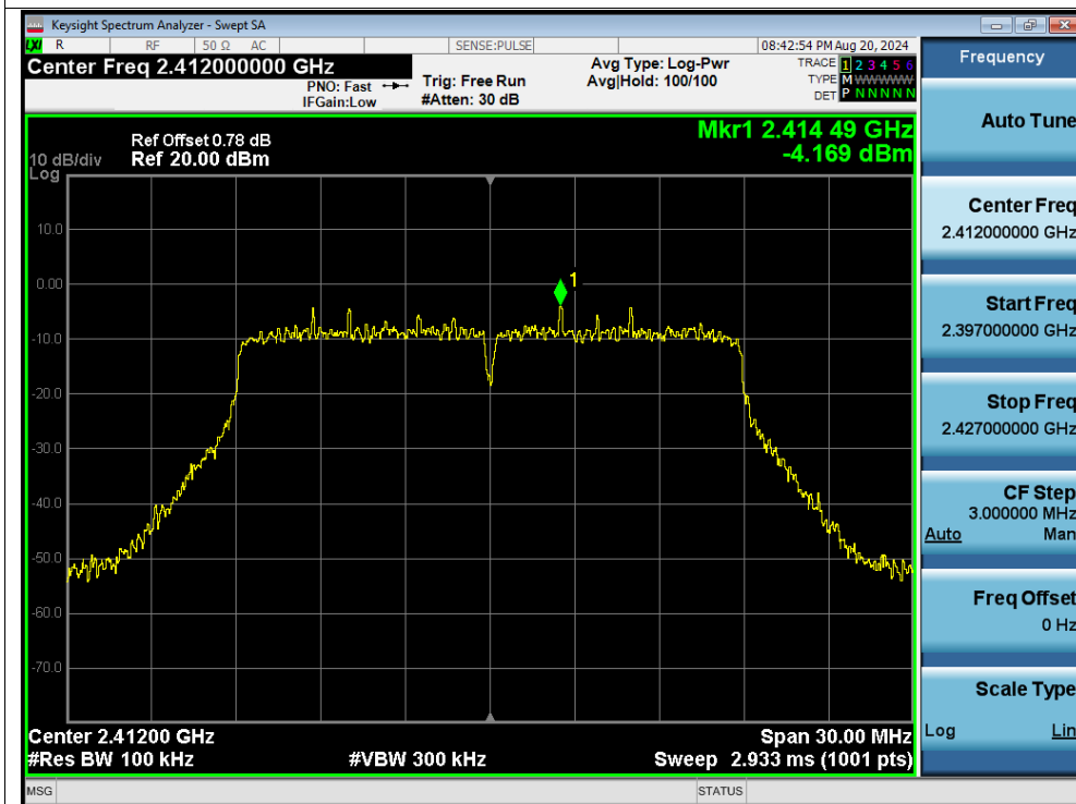
Band Edge NVNT n20 2412MHz Ant1 Emission
