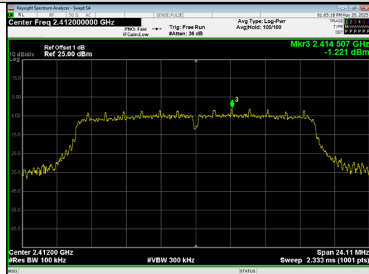
In-Band Reference Level IEEE 802.11g_Channel 1_20MHz_Antenna 0
