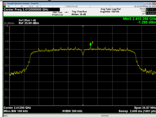
In-Band Reference Level IEEE 802.11n_Channel 1_20MHz_Antenna 0
