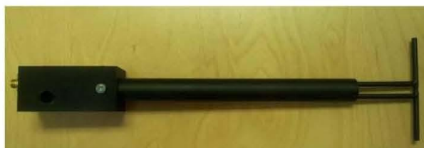
Figure 1 – MVG COMOSAR Validation Dipole
