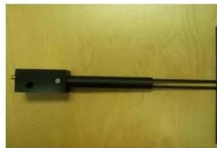
Figure 1 – MVG COMOSAR Validation Dipole
