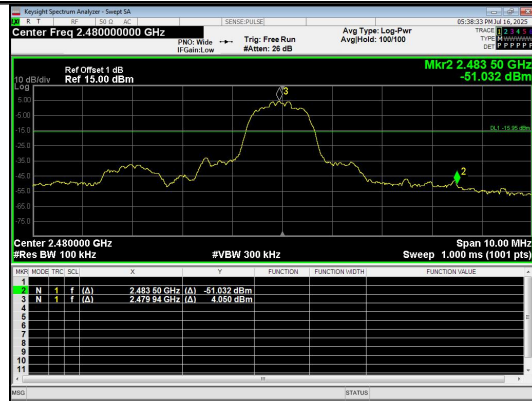
Out Of Band Emission 8DPSK_3-DH5_Channel 78
