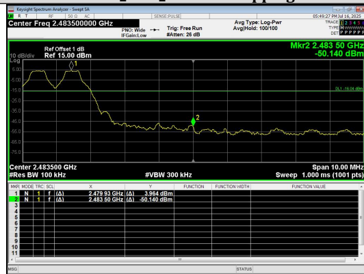
Out Of Band Emission(Right) GFSK_DH5_Channel Hopping
