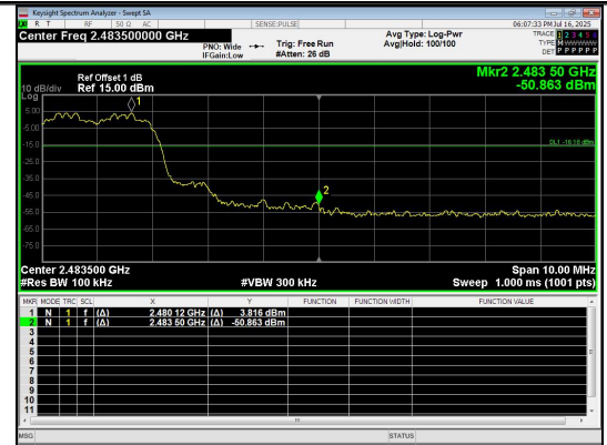
Out Of Band Emission(Right) 8DPSK_3-DH5_Channel Hopping
