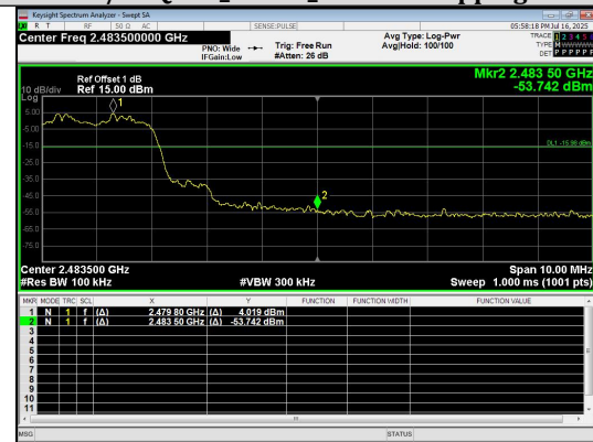
Out Of Band Emission(Right) \pi/4 DQPSK_2-DH5_Channel Hopping
