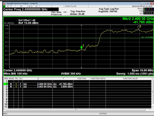
Out Of Band Emission(Left) 8DPSK_3-DH5_Channel Hopping
