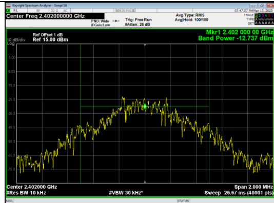
Peak Output Power 8DPSK_Channel 78
