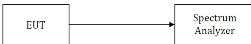
Test Setup Block Diagram
