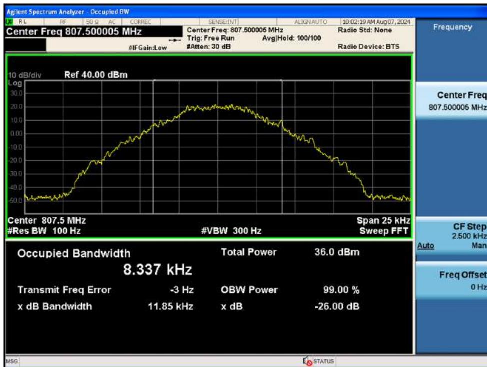
Input / B/ILT; SMR / 1 Carrier / Uplink / P25 Phase 1
