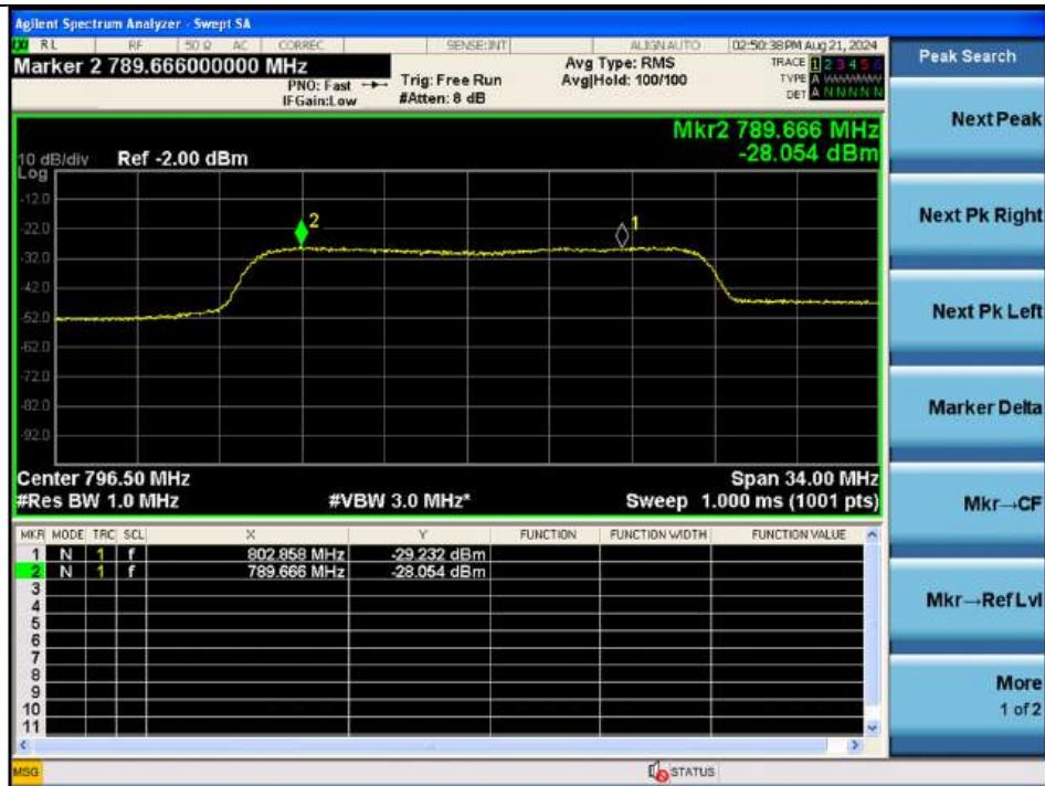
**Note:** The EUT is amplified over a frequency range of 788 ~ 806 MHz, but this test report uses the results for the frequency range of 788 ~ 798 MHz, 799 ~ 805 MHz.
