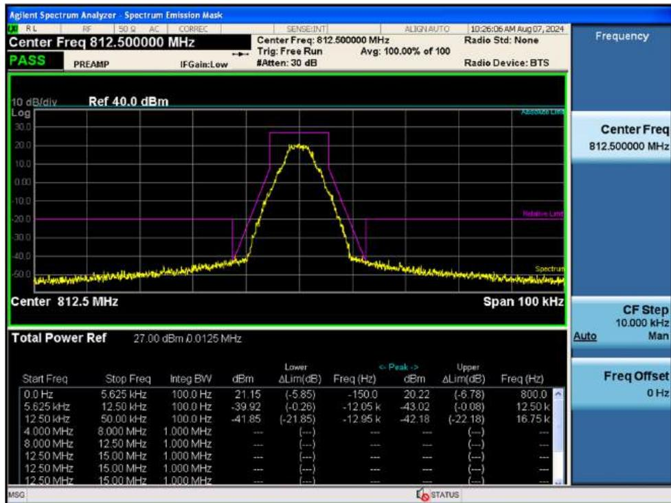
3 dB above the AGC threshold Input / B/ILT; SMR / 1 Carrier / Uplink / Mask D
