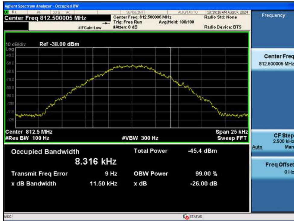
Output / B/ILT; SMR / 1 Carrier / Uplink / P25 Phase 1
