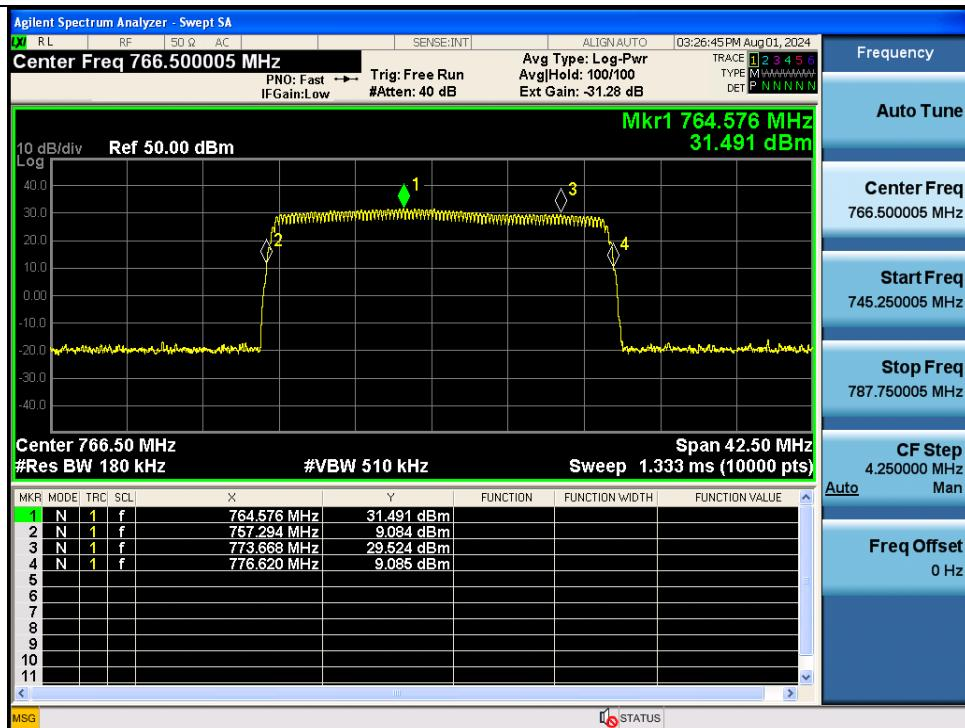
**Note:** The EUT is amplified over a frequency range of 758 ~ 776 MHz, but this test report uses the results for the frequency range of 758 ~ 768 MHz, 769 ~ 775 MHz.
