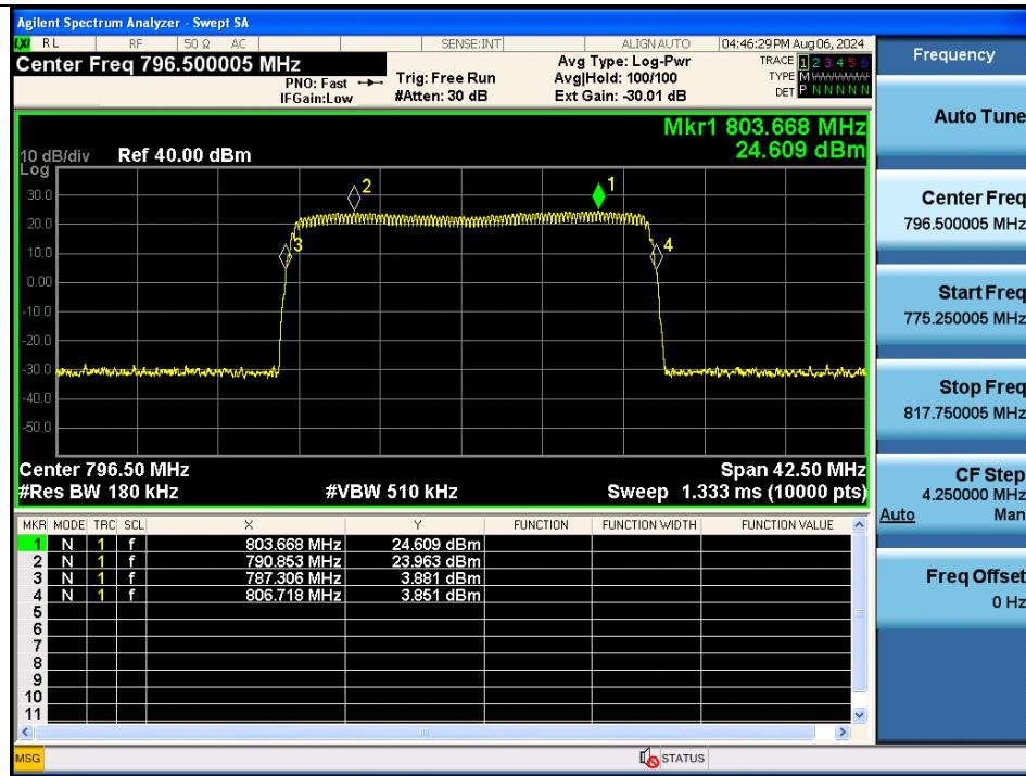
**Note:** The EUT is amplified over a frequency range of 788 ~ 806 MHz, but this test report uses the results for the frequency range of 799 ~ 805 MHz.
