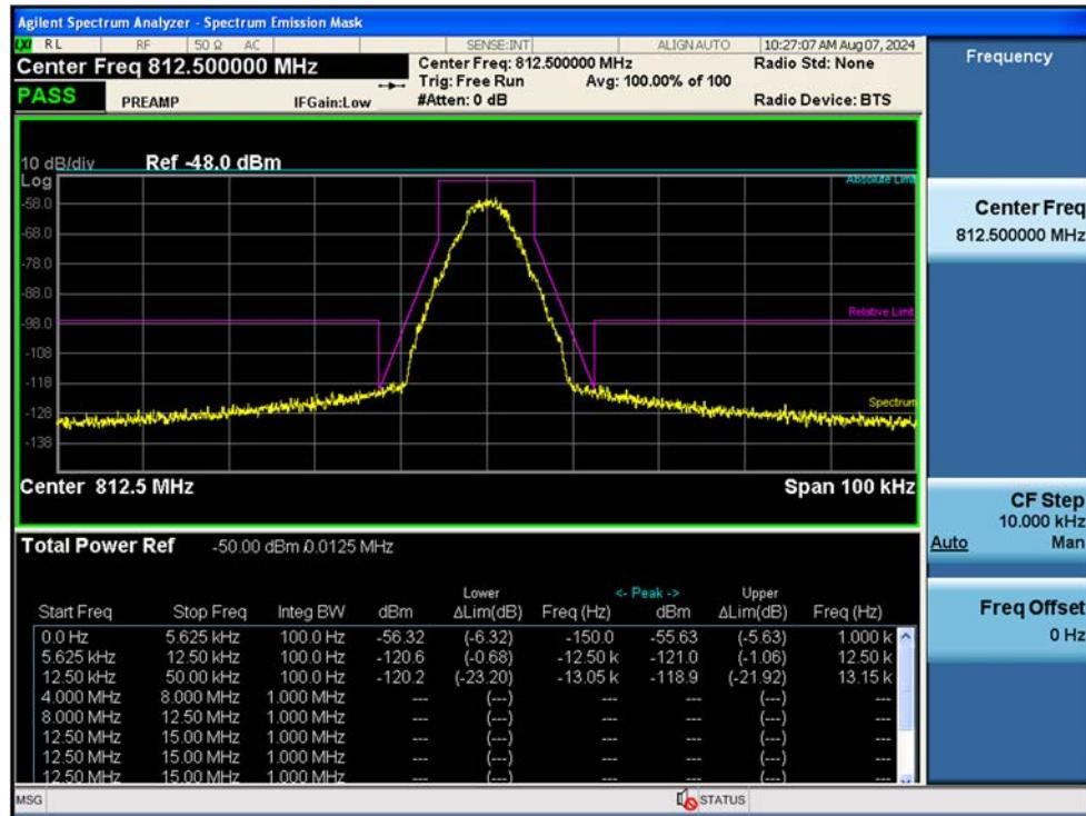
3 dB above the AGC threshold output / B/ILT; SMR / 1 Carrier / Uplink / Mask D
