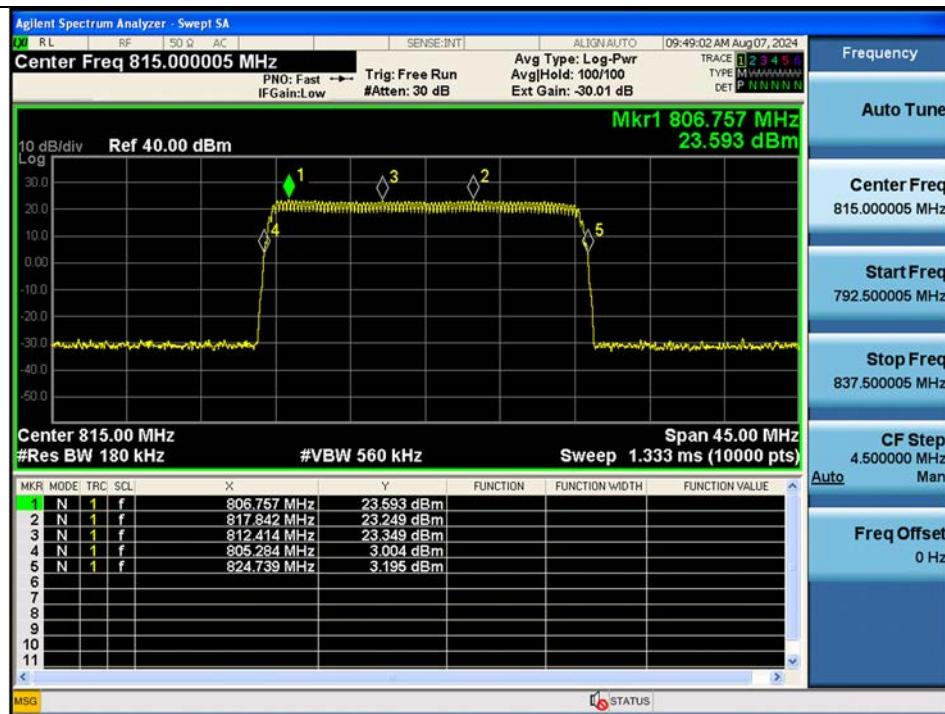
**Note:** The EUT is amplified over a frequency range of 806 ~ 824 MHz, but this test report uses the results for the frequency range of 806 ~ 809 MHz, 809 ~ 816 MHz, 817 ~ 824 MHz.
