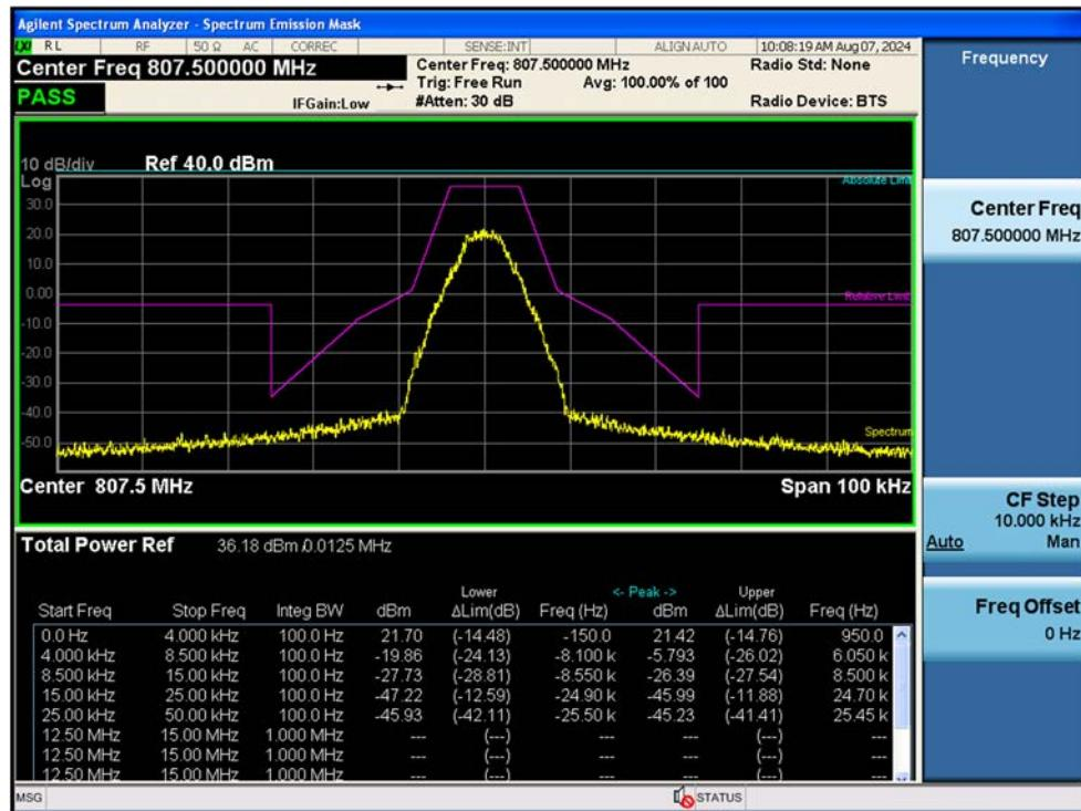
Input / B/ILT; SMR / 1 Carrier / Uplink / Mask D
