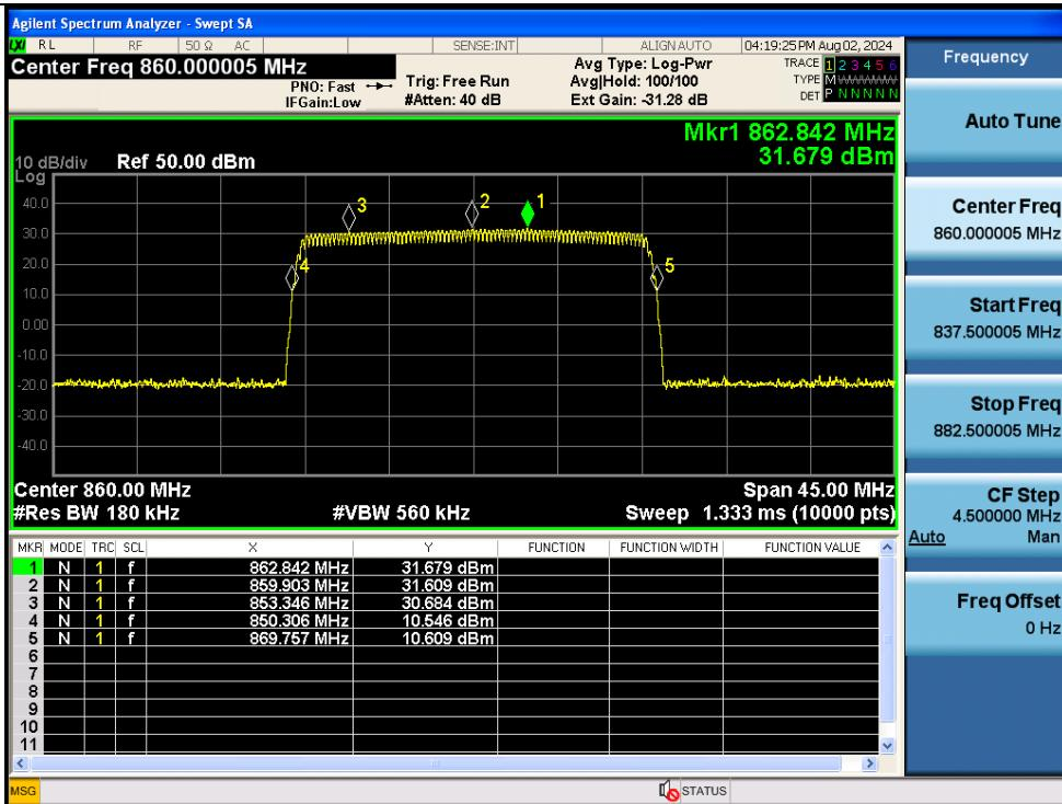
**Note:** The EUT is amplified over a frequency range of 851 ~ 869 MHz, but this test report uses the results for the frequency range of 851 ~ 854 MHz, 854 ~ 861 MHz, 862 ~ 869 MHz.
