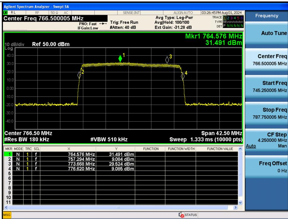
**Note:** The EUT is amplified over a frequency range of 758 ~ 776 MHz, but this test report uses the results for the frequency range of 769 ~ 775 MHz.
