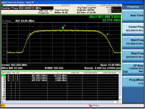
**Note:** The EUT is amplified over a frequency range of  $788 \sim 806$  MHz, but this test report uses the results for the frequency range of  $799 \sim 805$  MHz.
