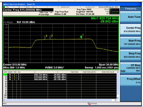
**Note:** The EUT is amplified over a frequency range of  $806 \sim 824$  MHz, but this test report uses the results for the frequency range of  $806 \sim 809$  MHz,  $809 \sim 816$  MHz,  $817 \sim 824$  MHz.
