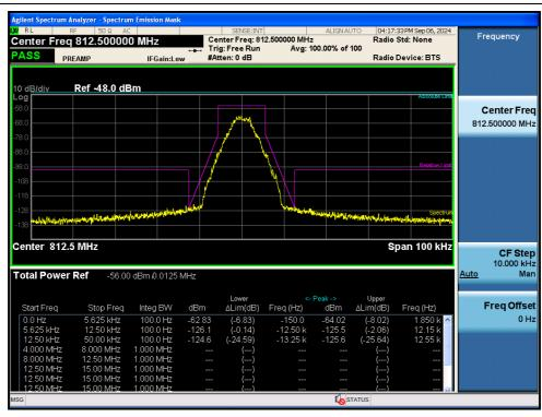
Input / B/ILT; SMR / 1 Carrier / Uplink / Mask D
