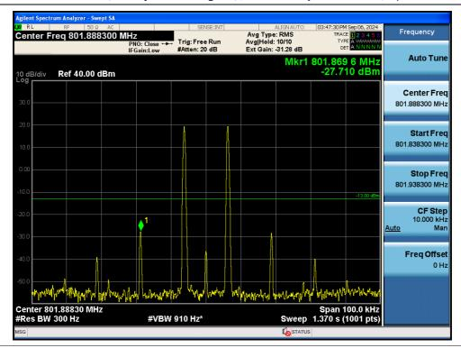
+3 dB above Out-of-band (two adjacent test signals) / Public Safety Narrowband / Uplink
