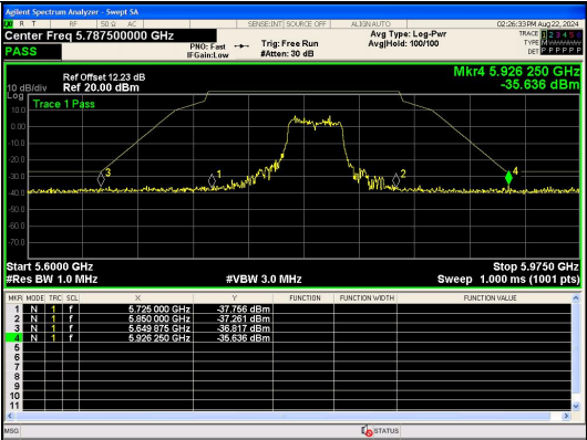
Out Of Band Emission IEEE 802.11ac_Channel 159_40MHz_Antenna 0
