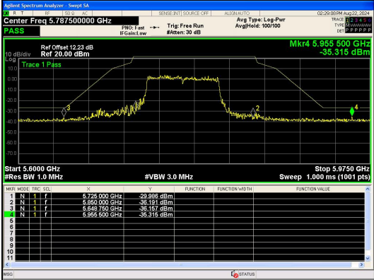
Out Of Band Emission IEEE 802.11ac_Channel 155_80MHz_Antenna 0
