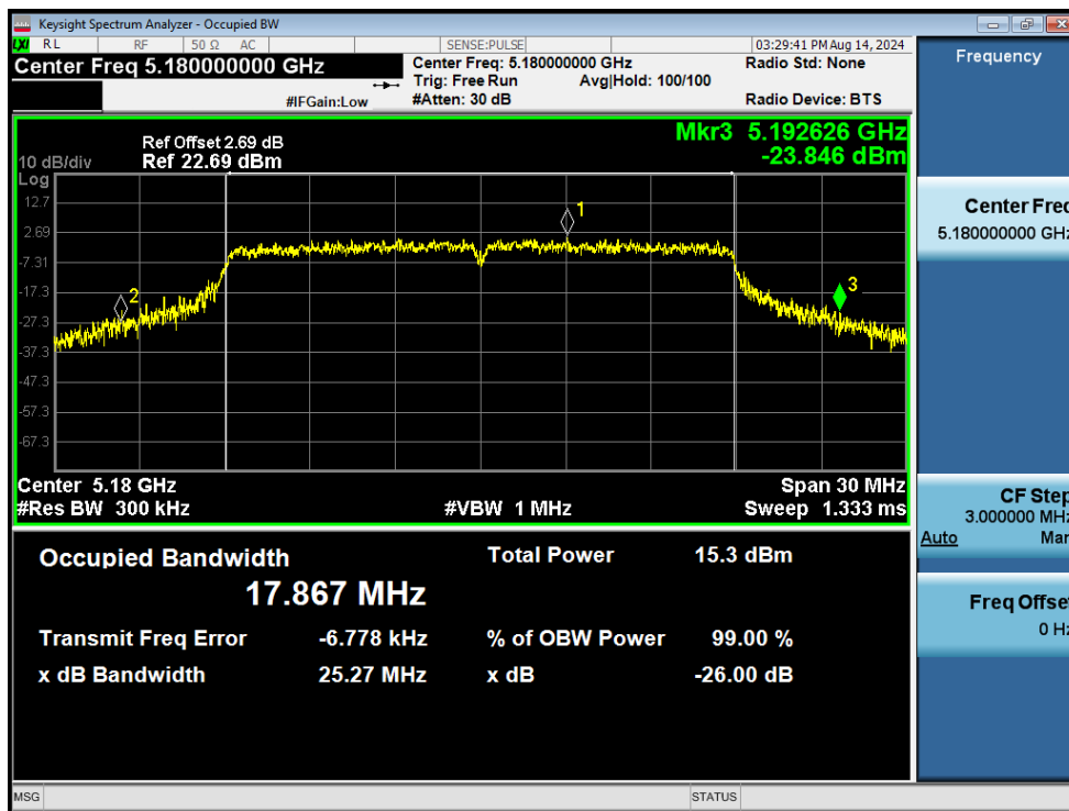
-26dB Bandwidth NVNT n20 5180MHz Ant1
