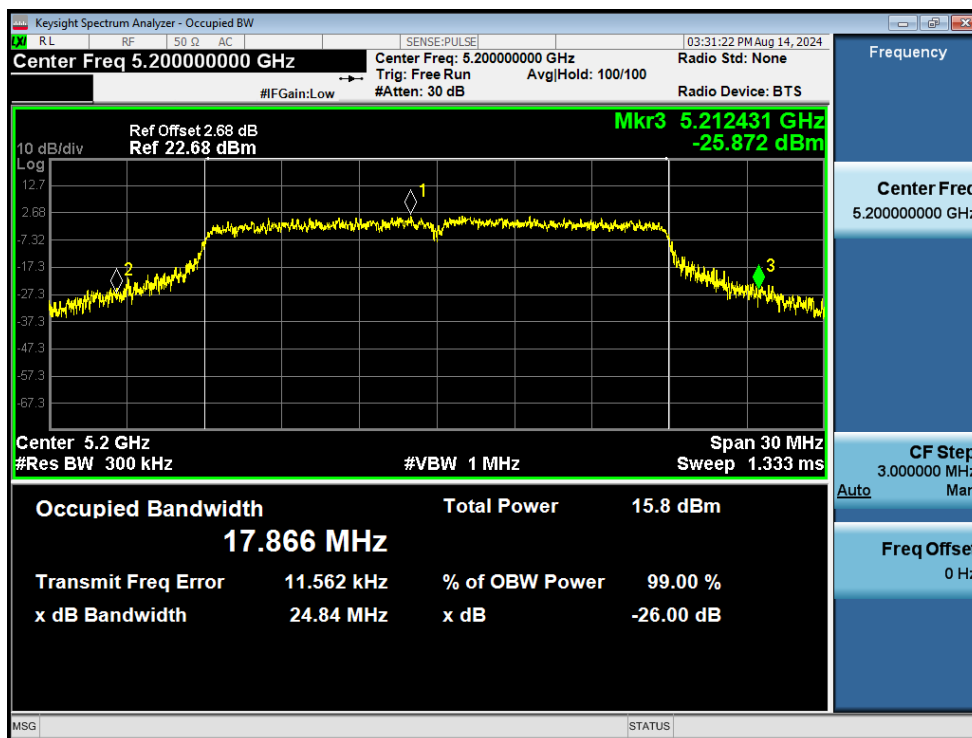
-26dB Bandwidth NVNT n20 5200MHz Ant1
