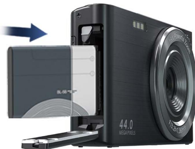
3. Keep the battery facing the same direction as the camera face as shown in the picture - (Installing the battery in the opposite direction will prevent charging), and then install the battery.
