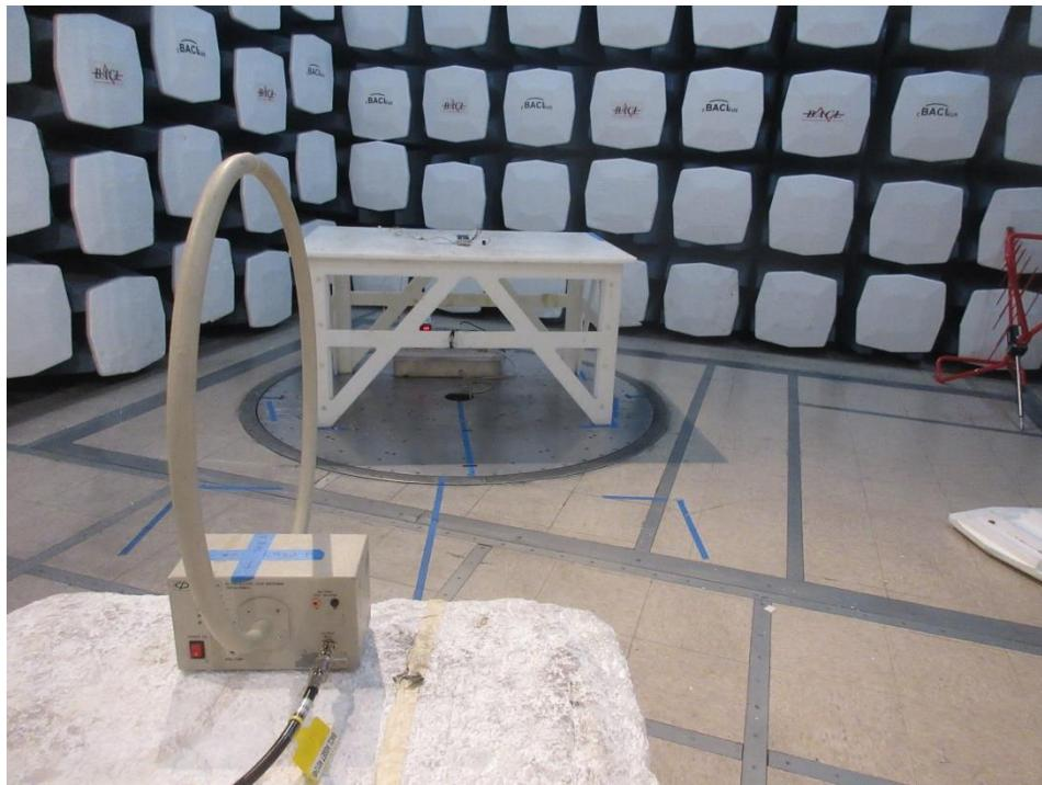
**1.4. EUT Test Setup at 3 Meters Loop Perpendicular Rear View (Below 30 MHz)**
