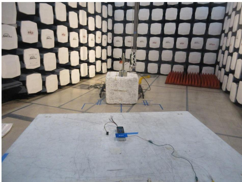
**1.5. EUT Test Setup at 3 Meters Front View (30 MHz – 150 MHz)**
