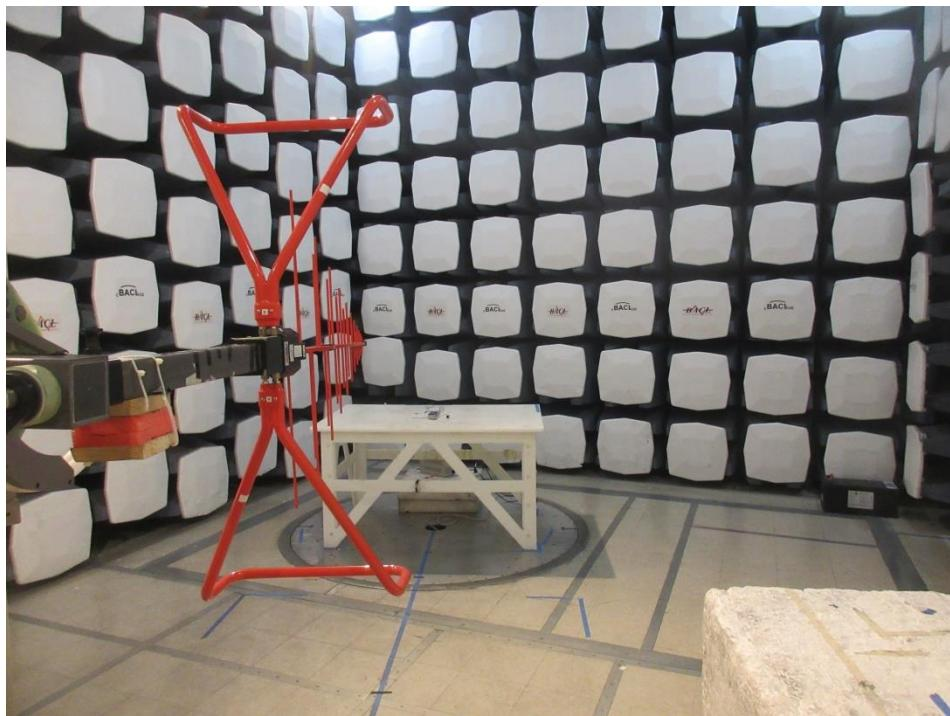
**1.6. EUT Test Setup at 3 Meters Rear View (30 MHz – 150 MHz)**
