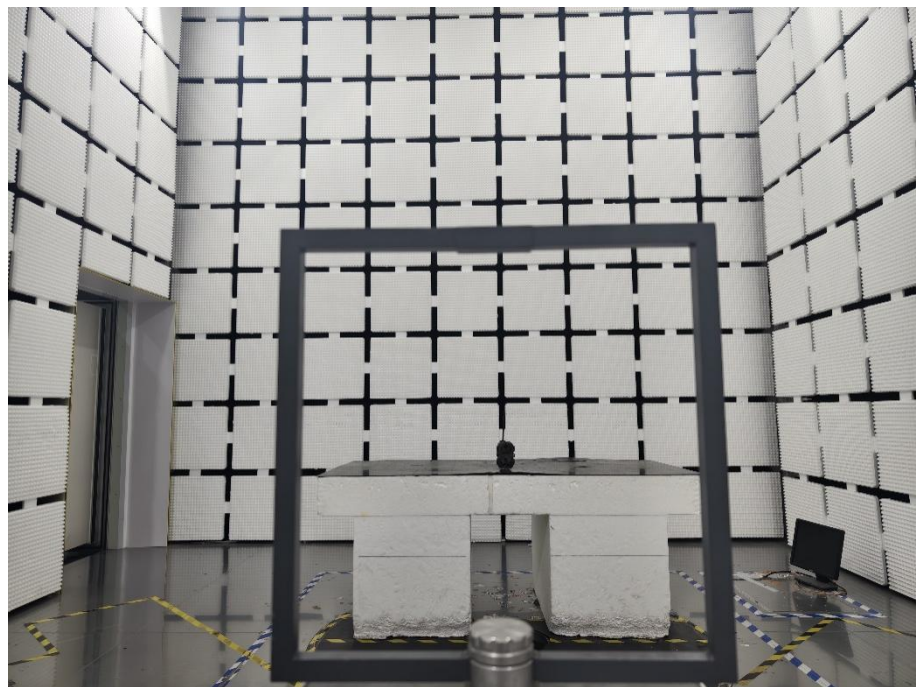
Radiation Emission Test Setup (Below 30MHz)
