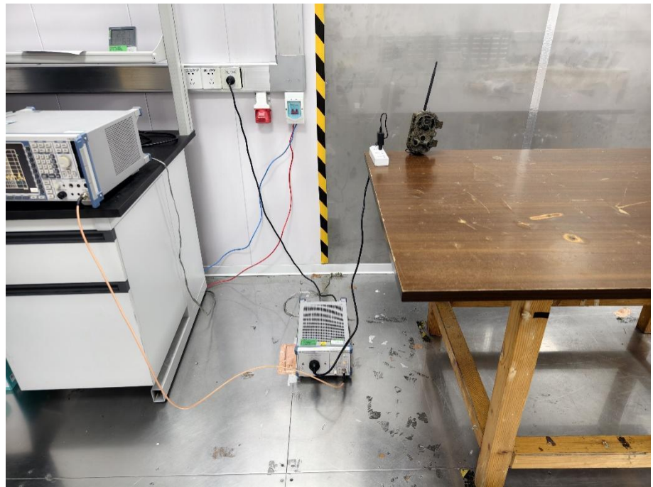
Conducted Emission Test Setup
