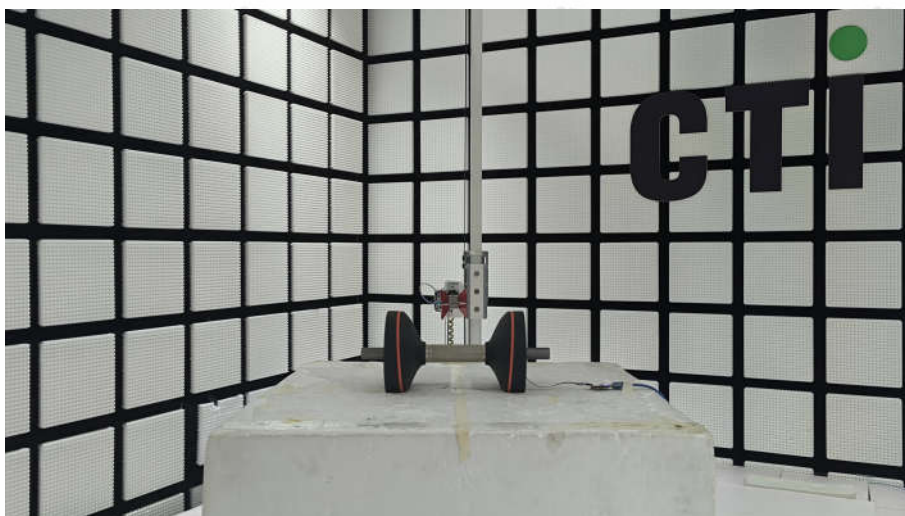
Radiated spurious emission Test Setup-2(Above 1GHz)
