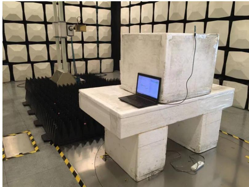
**Radiated Emission View (18GHz-25GHz)**
