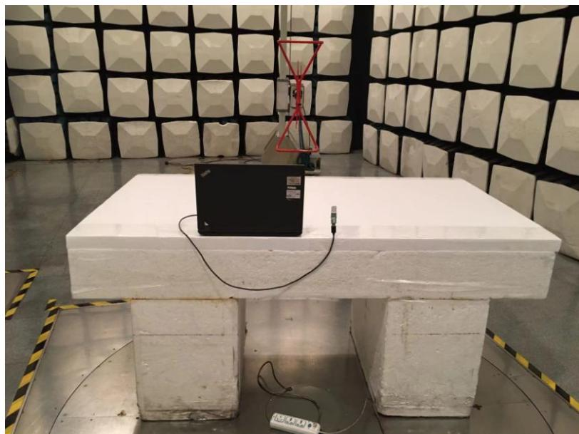
**Radiated Emission View (1GHz-18GHz)**
