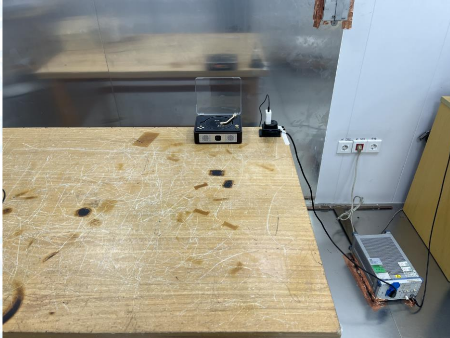
Photo of Setup for Conducted Emission
