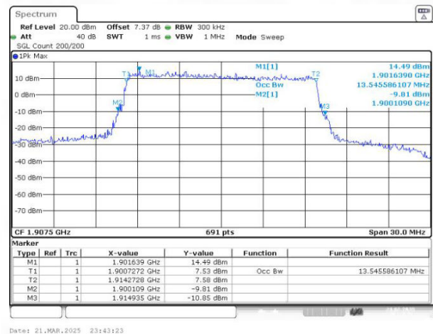
Band25 QAM16 BW=15MHz Channel=26615 RB Size=75 Position=#0
