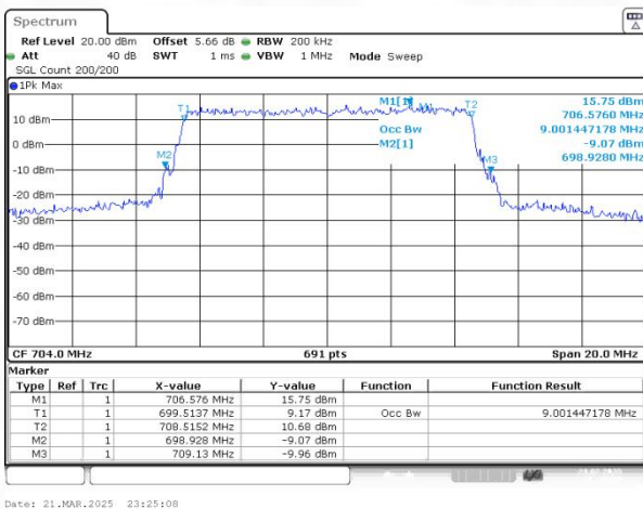
Band12 QPSK BW=10MHz Channel=23060 RB Size=50 Position=#0
