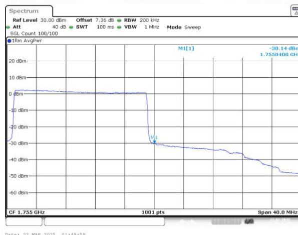
Band4 QPSK BW=20MHz Channel=20300 RB Size=100 Position=#0
