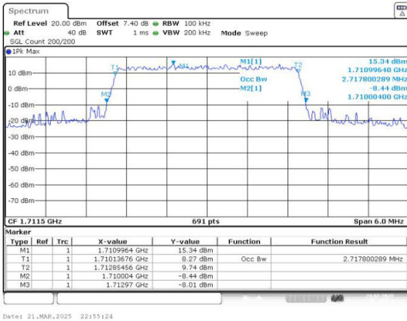
Band4 QAM16 BW=3MHz Channel=19965 RB Size=15 Position=#0
