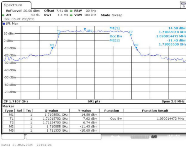
Band4 QPSK BW=1.4MHz Channel=19957 RB Size=6 Position=#0
