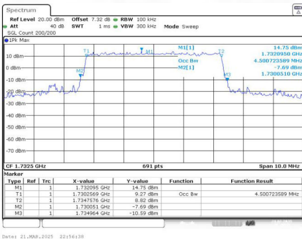
Band4 QAM16 BW=5MHz Channel=20175 RB Size=25 Position=#0
