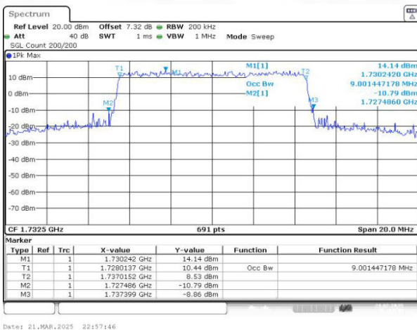
Band4 QAM16 BW=10MHz Channel=20175 RB Size=50 Position=#0
