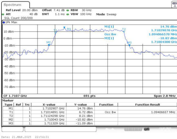
Band4 QAM16 BW=1.4MHz Channel=19957 RB Size=6 Position=#0
