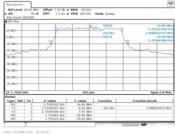
Band4 QAM16 BW=1.4MHz Channel=20175 RB Size=6 Position=#0
