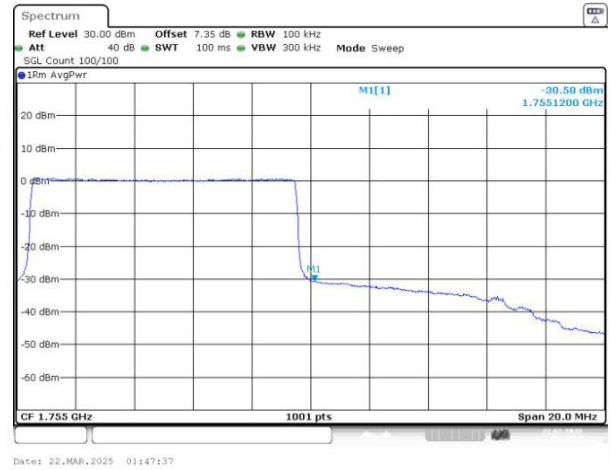
Band4 QAM16 BW=10MHz Channel=20350 RB Size=50 Position=#0
