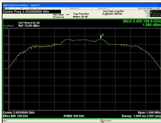
In-Band Reference Level 8DPSK_3-DH1_Channel 0
