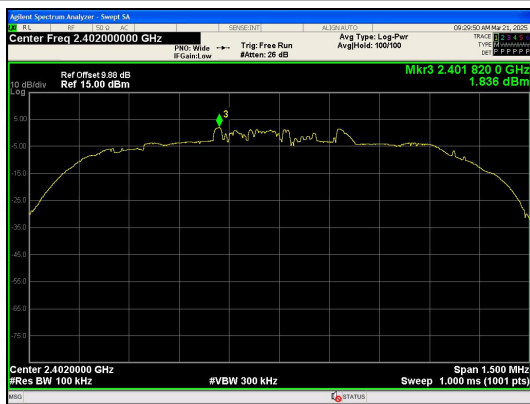
In-Band Reference Level 8DPSK_3-DH5_Channel 0
