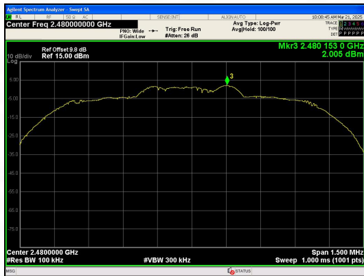
In-Band Reference Level \pi/4 DQPSK_2-DH3_Channel 78
