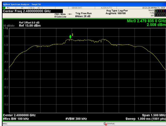
In-Band Reference Level 8DPSK_3-DH1_Channel 78
