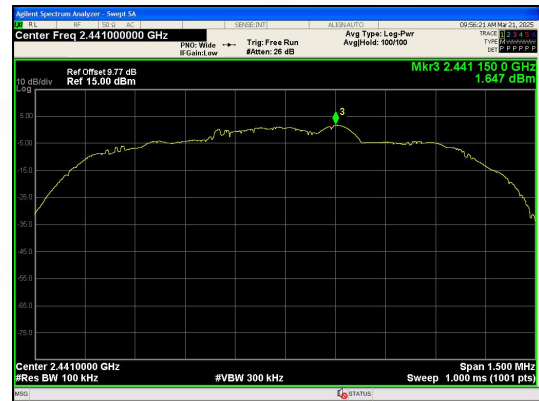
In-Band Reference Level 8DPSK_3-DH3_Channel 39
