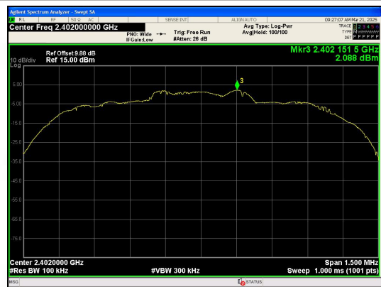
In-Band Reference Level 8DPSK_3-DH3_Channel 0
