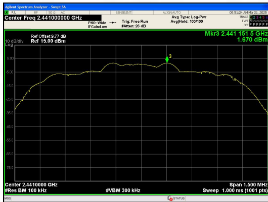
In-Band Reference Level 8DPSK_3-DH1_Channel 39
