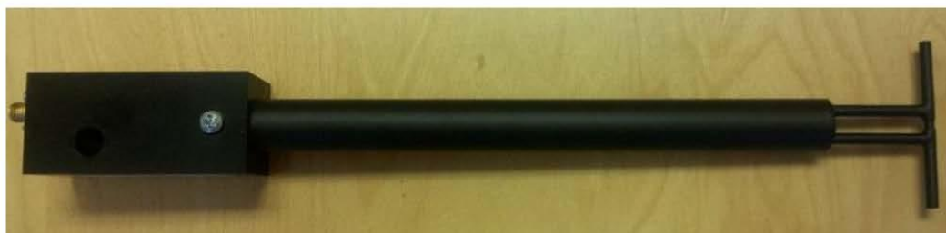
Figure 1 – MVG COMOSAR Validation Dipole
