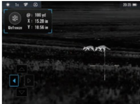
When the reticle is aligned with the point of impact, press and hold the MENU button to save and exit. You can also press the POWER button, a window will pop up to prompt whether to save. Press the UP button to exit with saving or the DOWN button to exit without saving.
