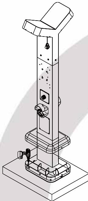
Align the screw holes of the pedestal with the ones in the concrete pier
