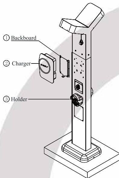
Assemble the backplate on the pedestal as explained in Section 8.6
