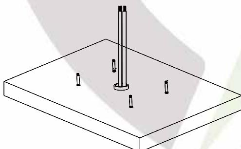
Drive the expansion screw into the concrete pier
