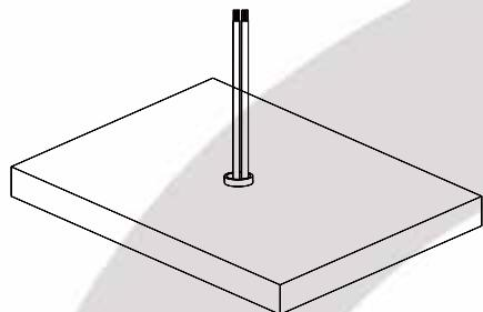
Build a concrete pier on the ground (17.72" x 13.78" x 7.87")
