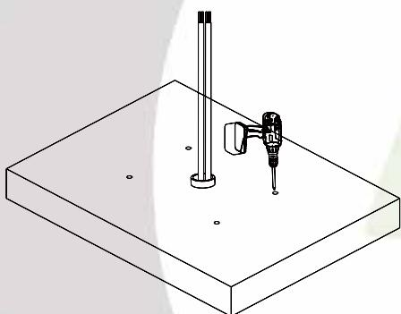
Draw one cable (two cables for dual chargers) from the center
