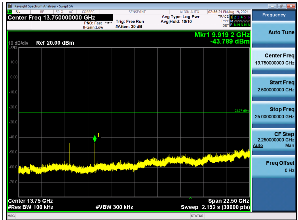
Test_Graph_LE1M_ANT1_2480_1Mbps_Higher Band Emissions
