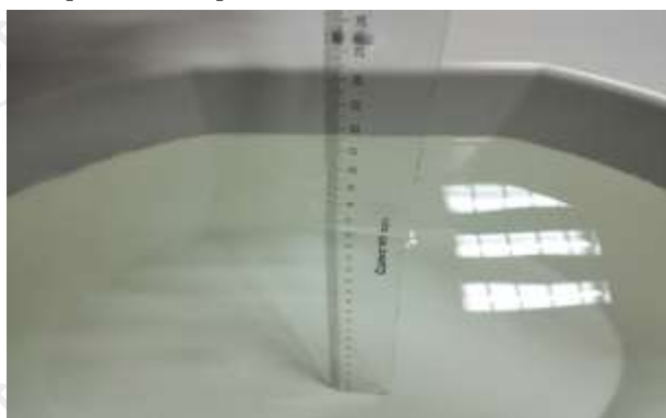
The Body Liquid of 5000-6000MHz (16.5cm)
