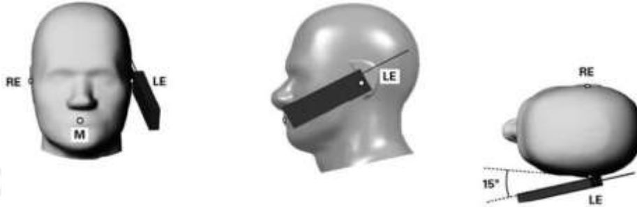
Positioning for Ear / 15° Tilt
