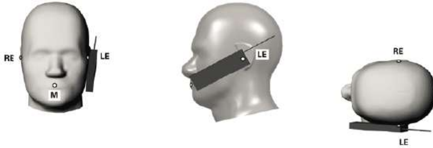
Positioning for Ear / 15° Tilt
