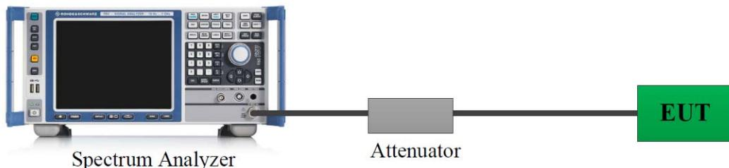
A short RF cable with low cable loss connected to the EUT antenna port, which was provided by manufacturer.
