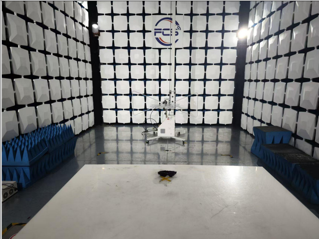
Above 1GHz for radiated emission test setup
