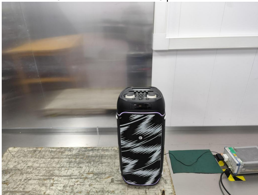
Conducted Emission at AC power line
