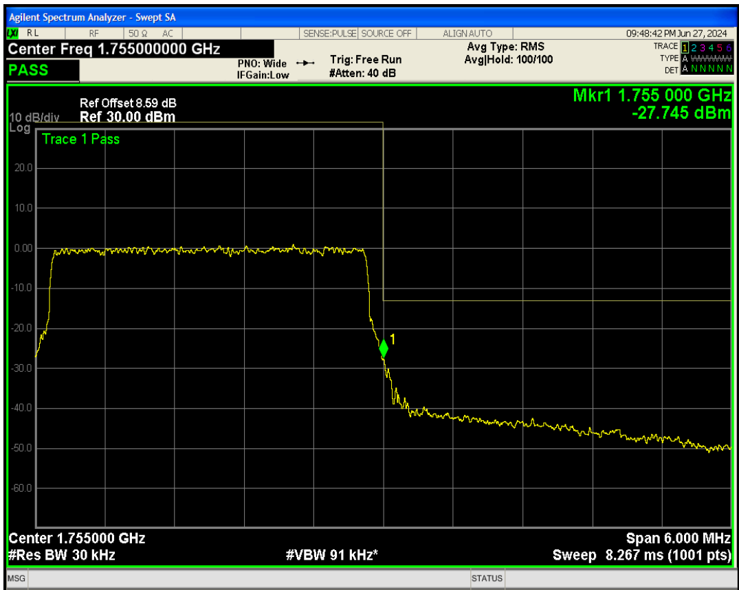
Band4 QPSK BW=5MHz Channel=19975 RB Size=25 Position=#0
