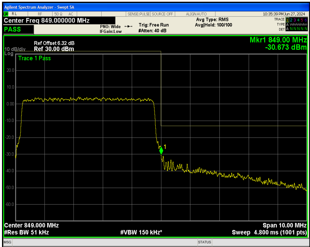
Band5 QPSK BW=10MHz Channel=20450 RB Size=50 Position=#0
