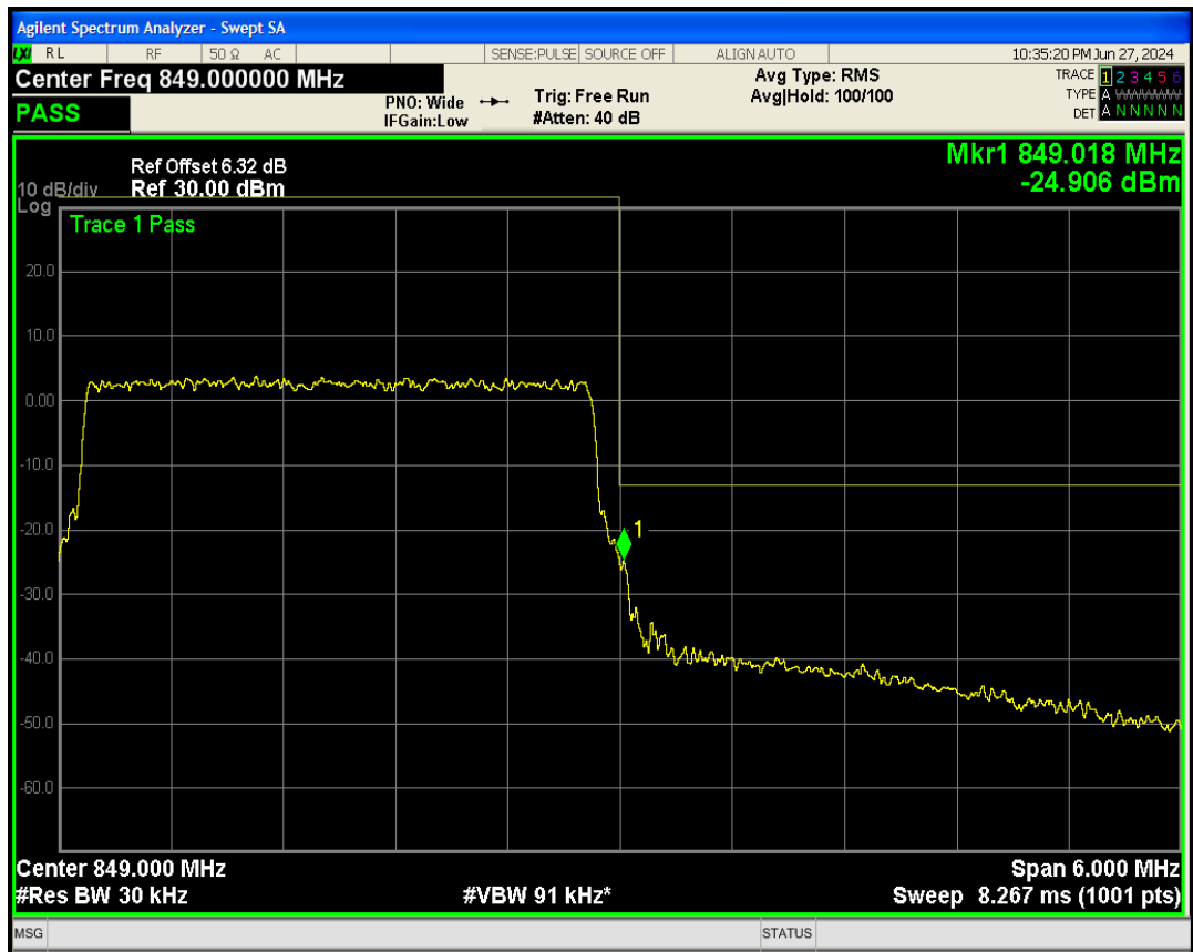
Band5 QAM16 BW=5MHz Channel=20425 RB Size=25 Position=#0
