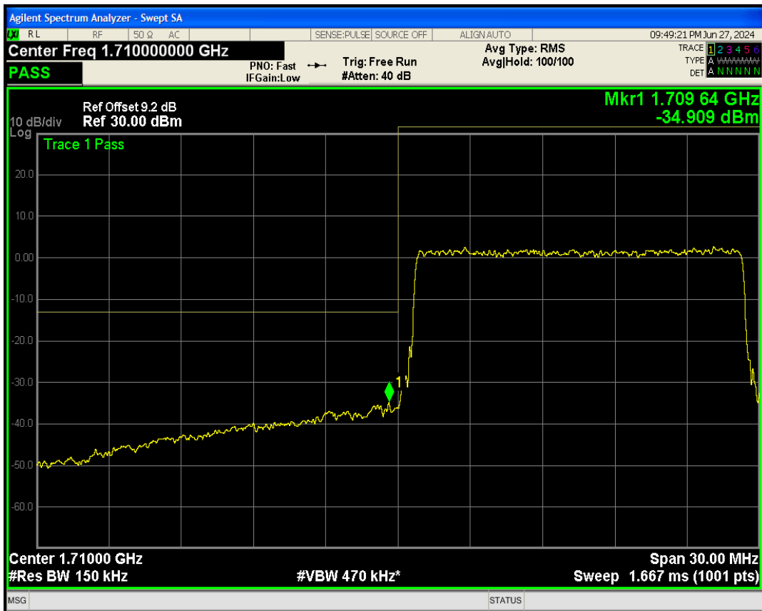
Band4 QAM16 BW=15MHz Channel=20025 RB Size=75 Position=#0
