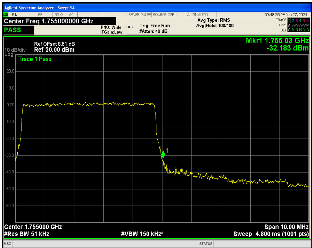
Band4 QAM16 BW=5MHz Channel=20375 RB Size=25 Position=#0
