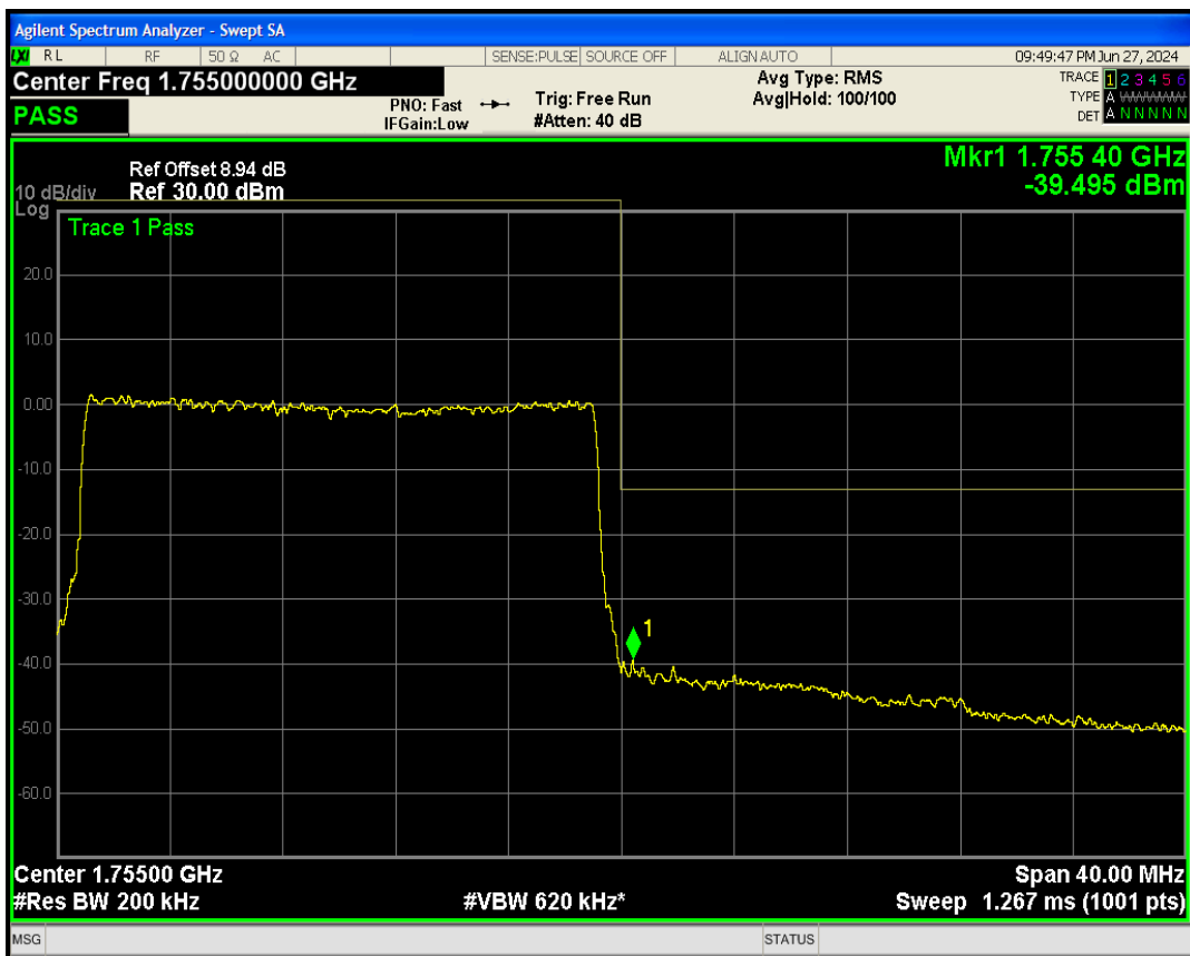
Band4 QPSK BW=20MHz Channel=20300 RB Size=100 Position=#0
