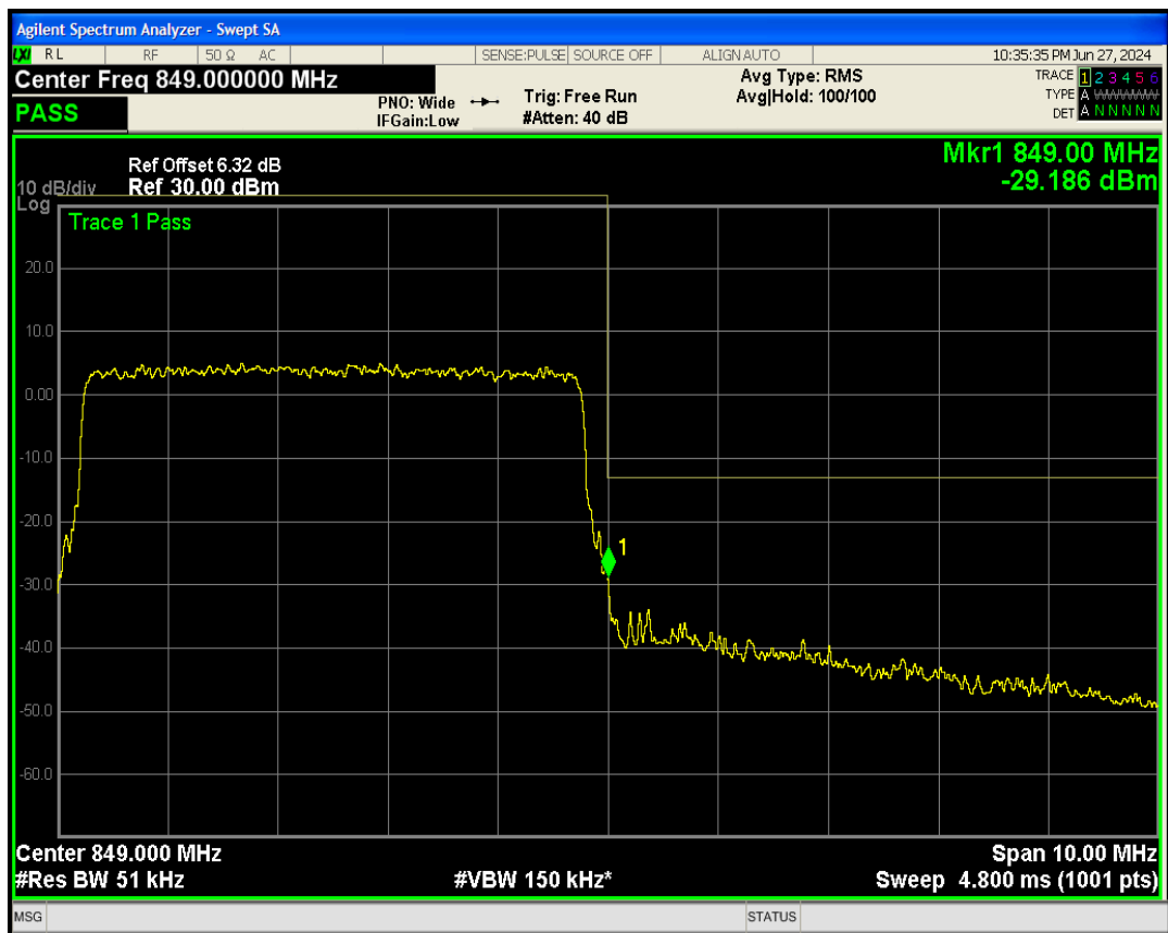
Band5 QAM16 BW=5MHz Channel=20625 RB Size=25 Position=#0
