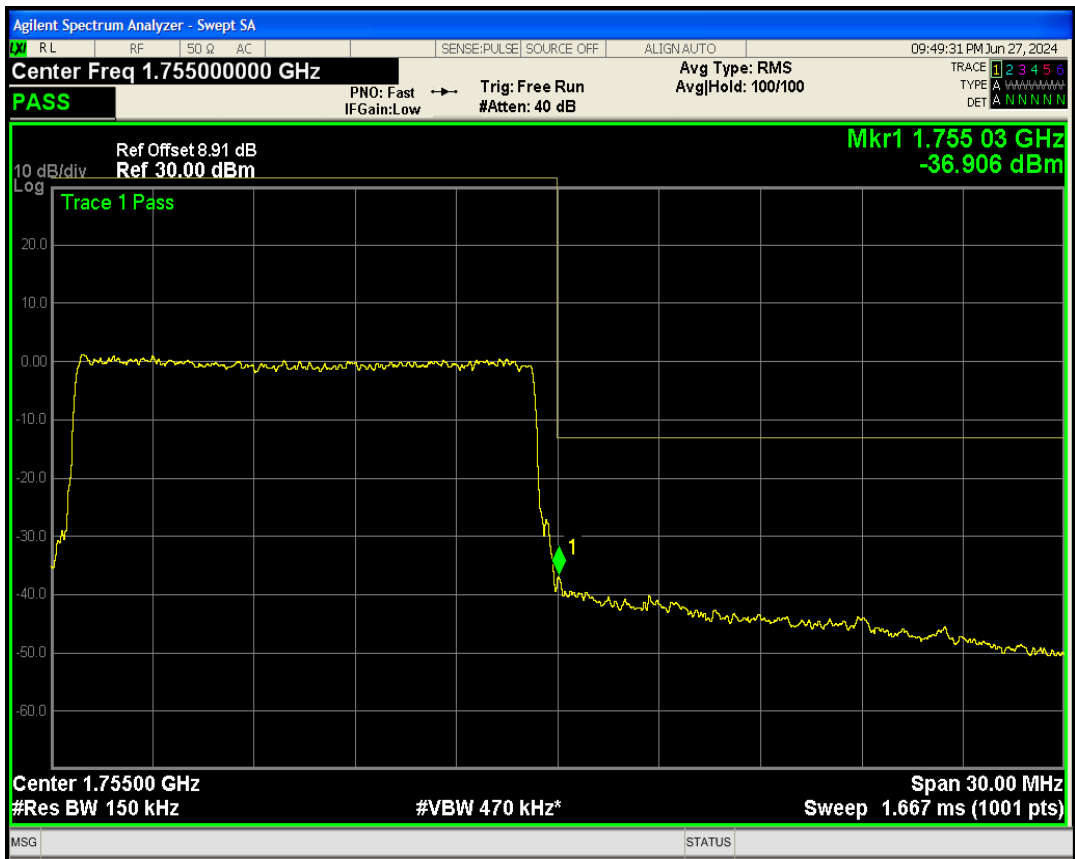
Band4 QPSK BW=20MHz Channel=20050 RB Size=100 Position=#0
