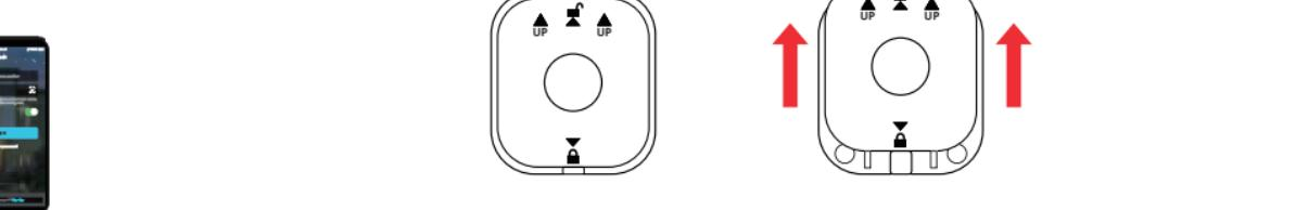
2. Once you have confirmed the cameras mounting location, we recommend installation to be at a height of 9ft to maximize the Ai detection ability.
