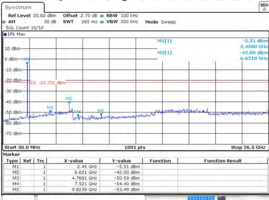
**Tx. Spurious NVNT n20 2412MHz Ant1 Ref**
