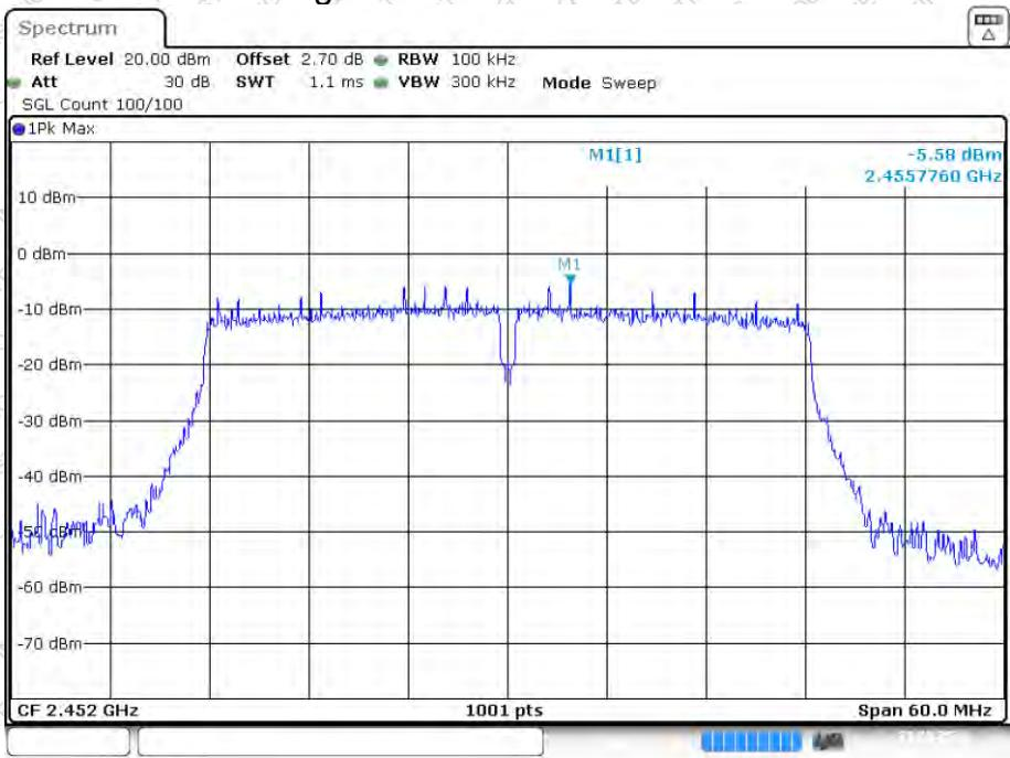
**Band Edge NVNT n40 2452MHz Ant1 Emission**
