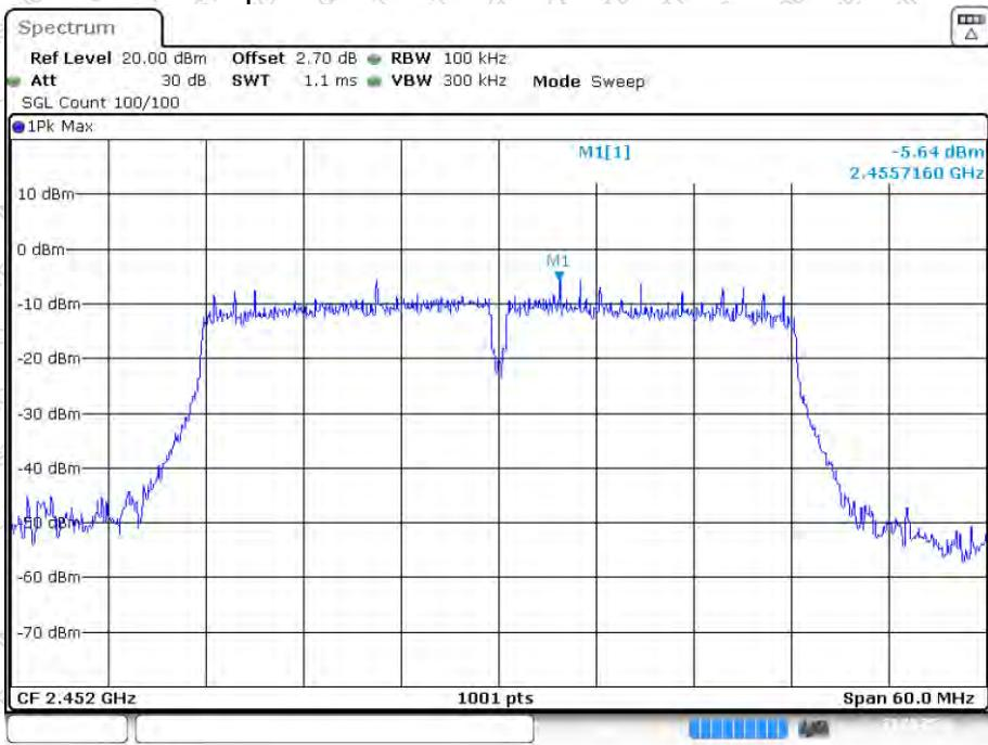
**Tx. Spurious NVNT n40 2452MHz Ant1 Emission**
