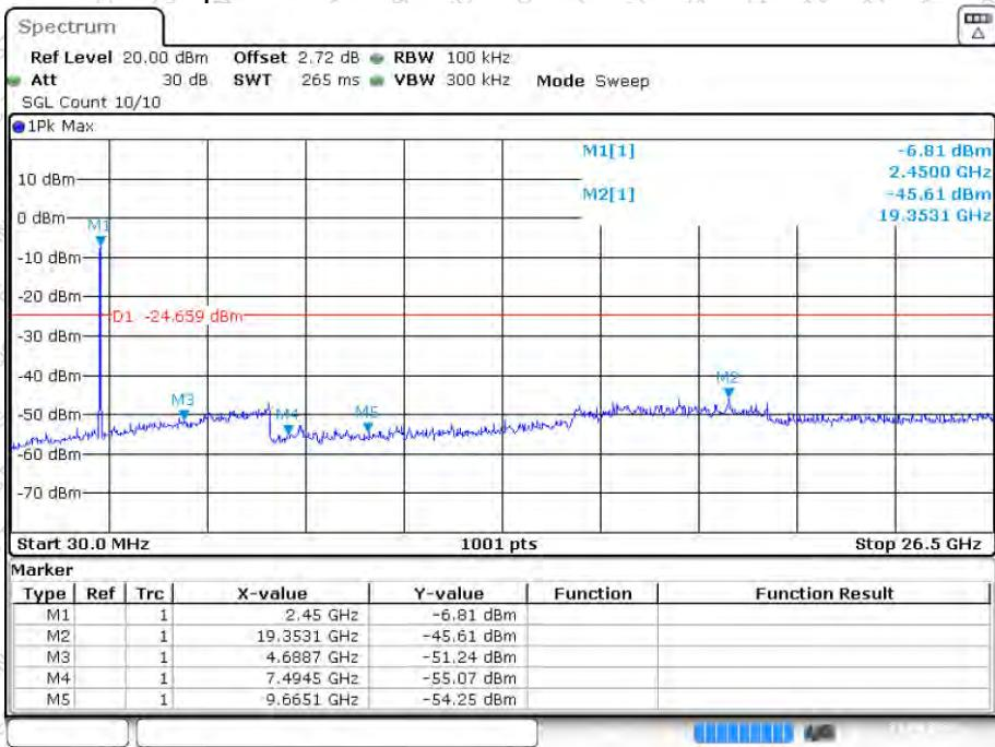
**Tx. Spurious NVNT n40 2452MHz Ant1 Ref**
