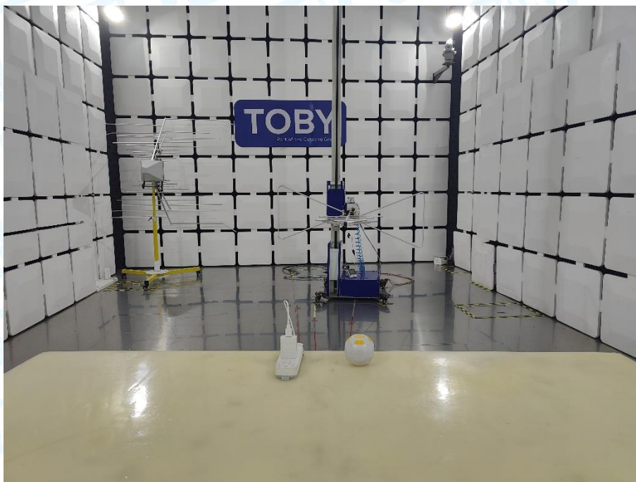
Photo of Setup for Radiated Emission (30MHz~1GHz)
