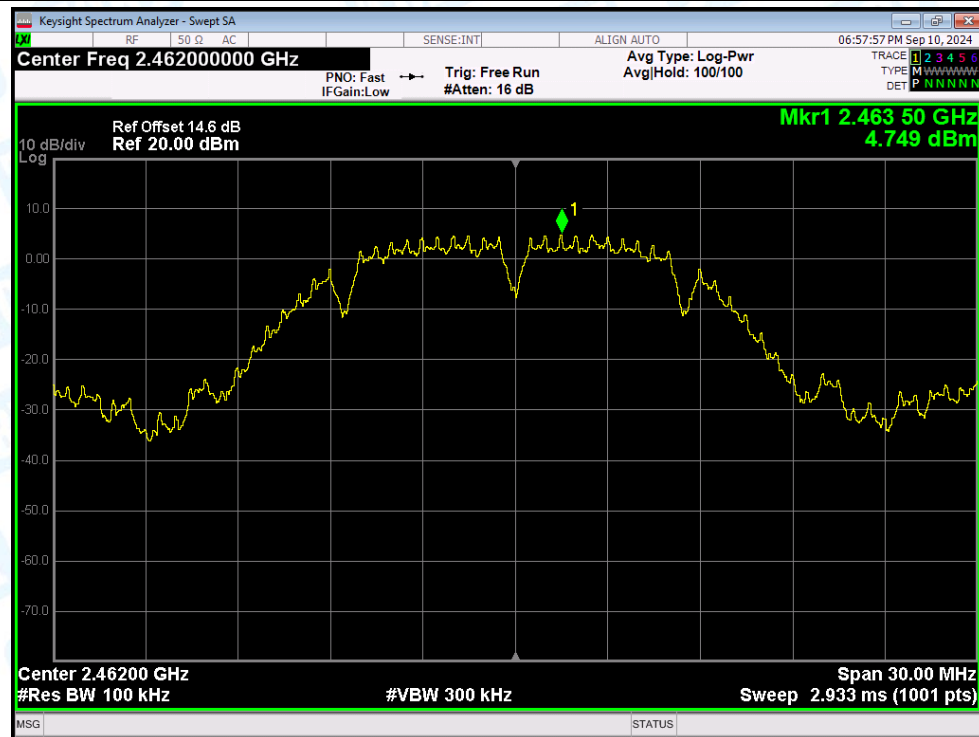
Tx. Spurious NVNT b 2462MHz Ant1 Emission
