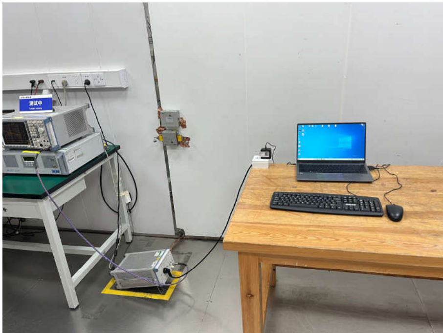
Conducted Emissions Test Setup
