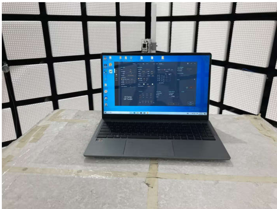
Radiated spurious emission Test Setup-3(Above 18GHz)
