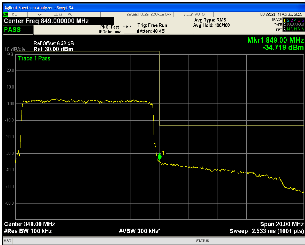
Band66 QPSK BW=1.4MHz Channel=131979 RB Size=6 Position=#0
