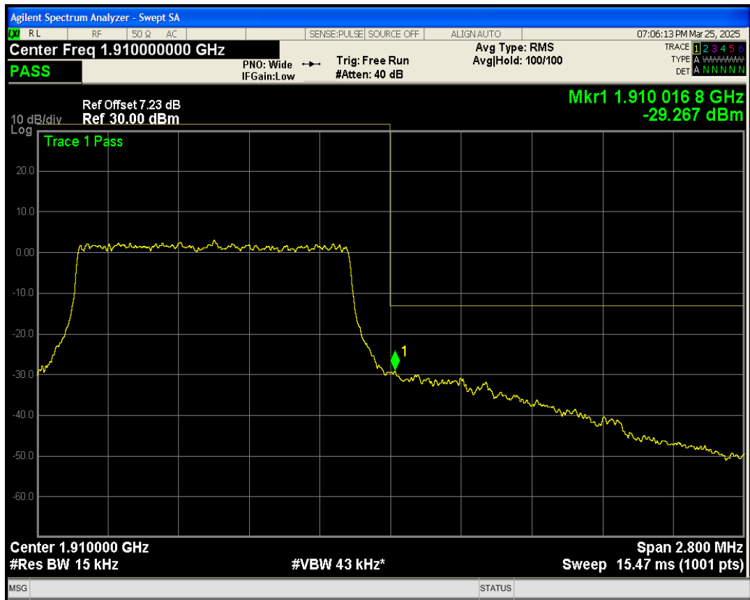
Band2 QAM16 BW=3MHz Channel=18615 RB Size=15 Position=#0
