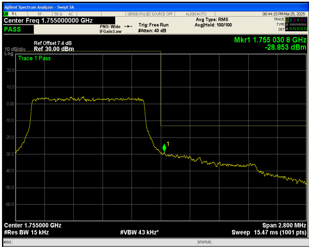
Band4 QPSK BW=3MHz Channel=19965 RB Size=15 Position=#0
