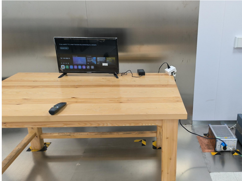
Radiated Emission Test View|(Below 1G)
