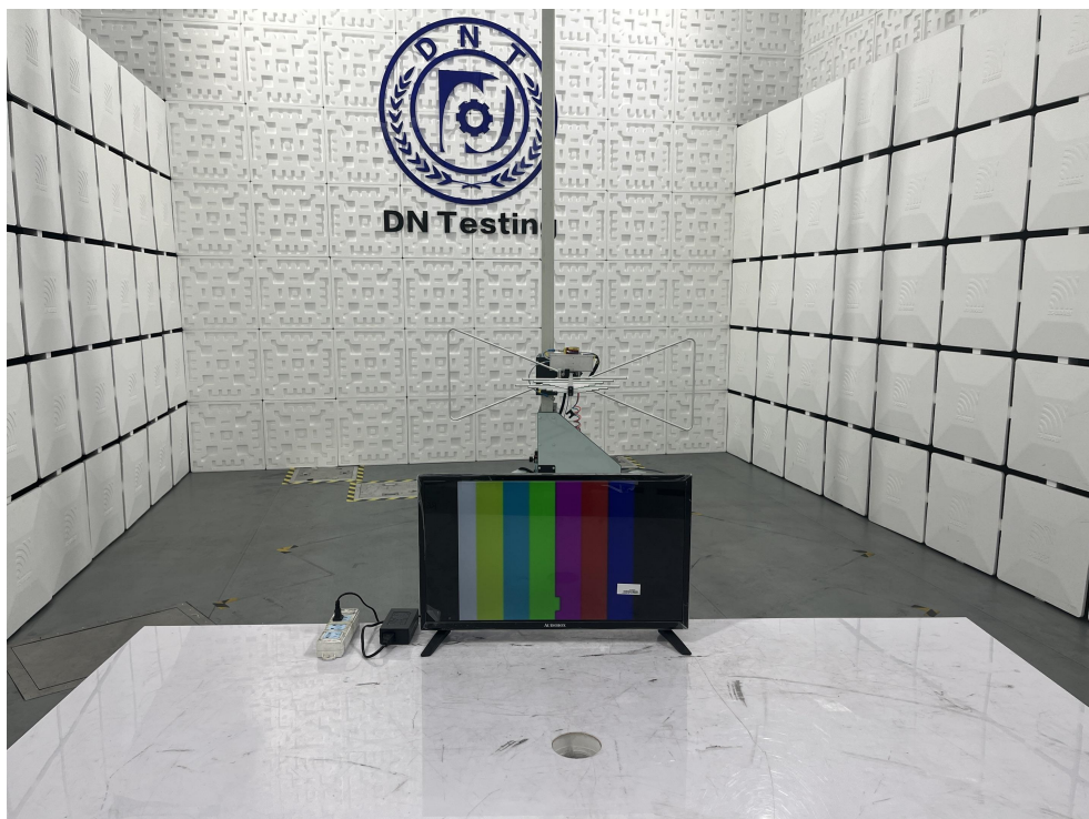
Radiated Emission Test View|(Below 1G)
