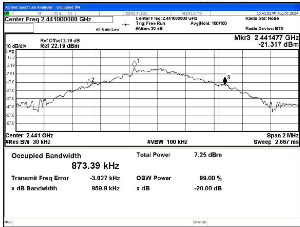
-20dB Bandwidth NVNT 1-DH5 2441MHz Ant1
