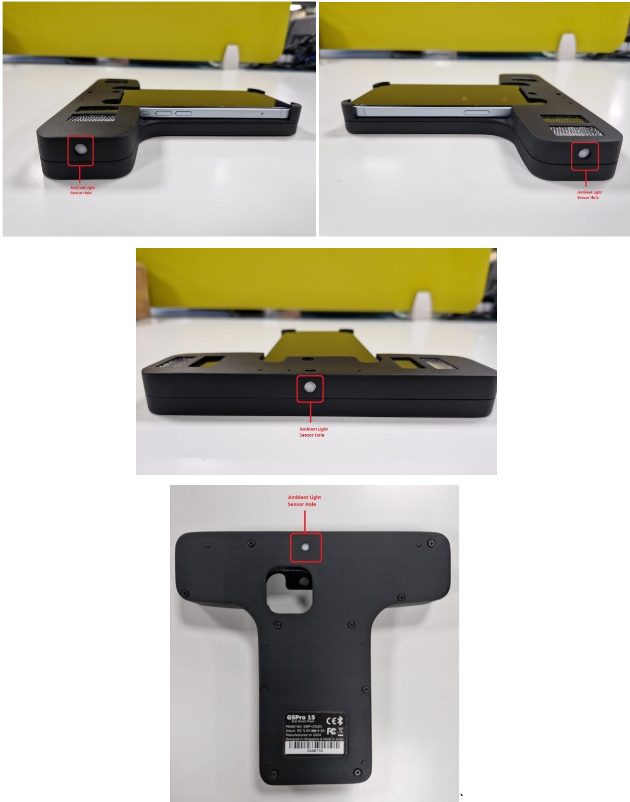
Fig 3: Ambient Light Sensor Hole in the enclosure
