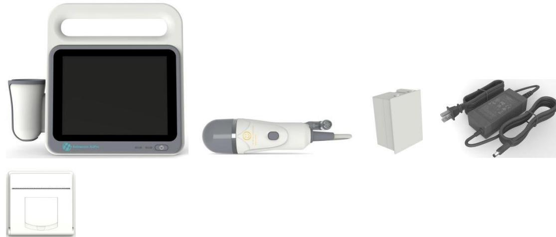
The console showcases critical information such as ultrasonic images, bladder volume values, and offers the majority of the control. The lithium-ion battery pack is accountable for the power supply and can be charged via the console when a supply mains is connected using a medical switching power supply. The built-in printer can print bladder scan reports and self-test reports. The probe is utilized to scan the patient bladder.
