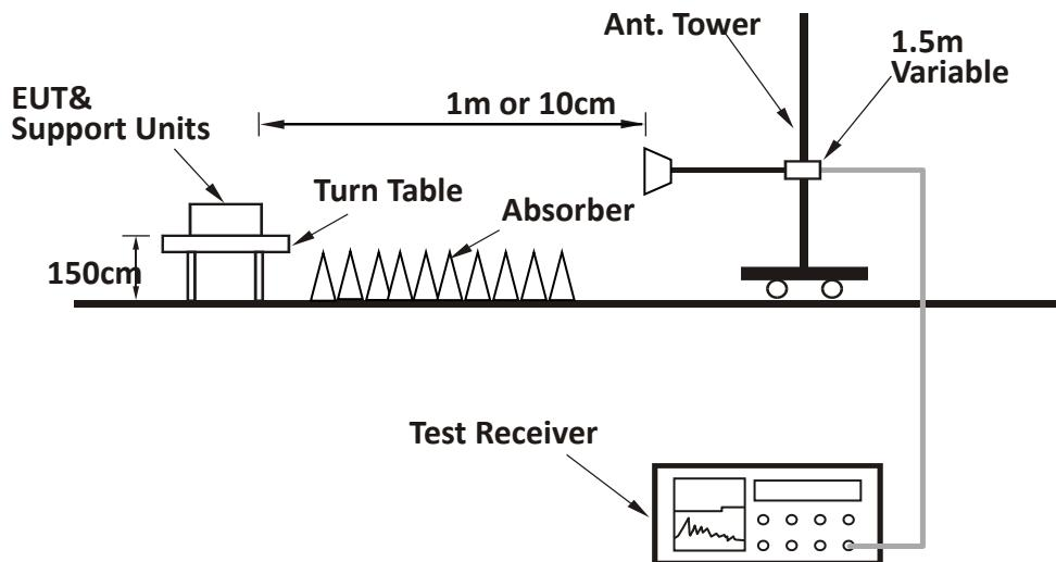
**TEST REPORT****4.4 Test Results of Radiated Emissions**
