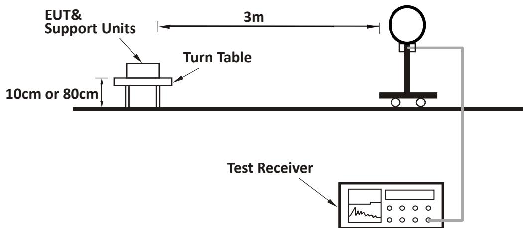
**For Radiated emission 30MHz to 1GHz:**
