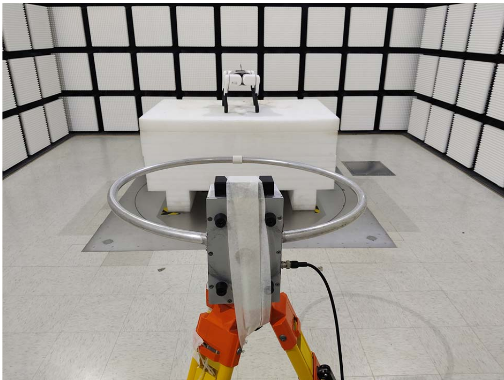
Radiated Emission 9 kHz-30 MHz Ground-parallel View
