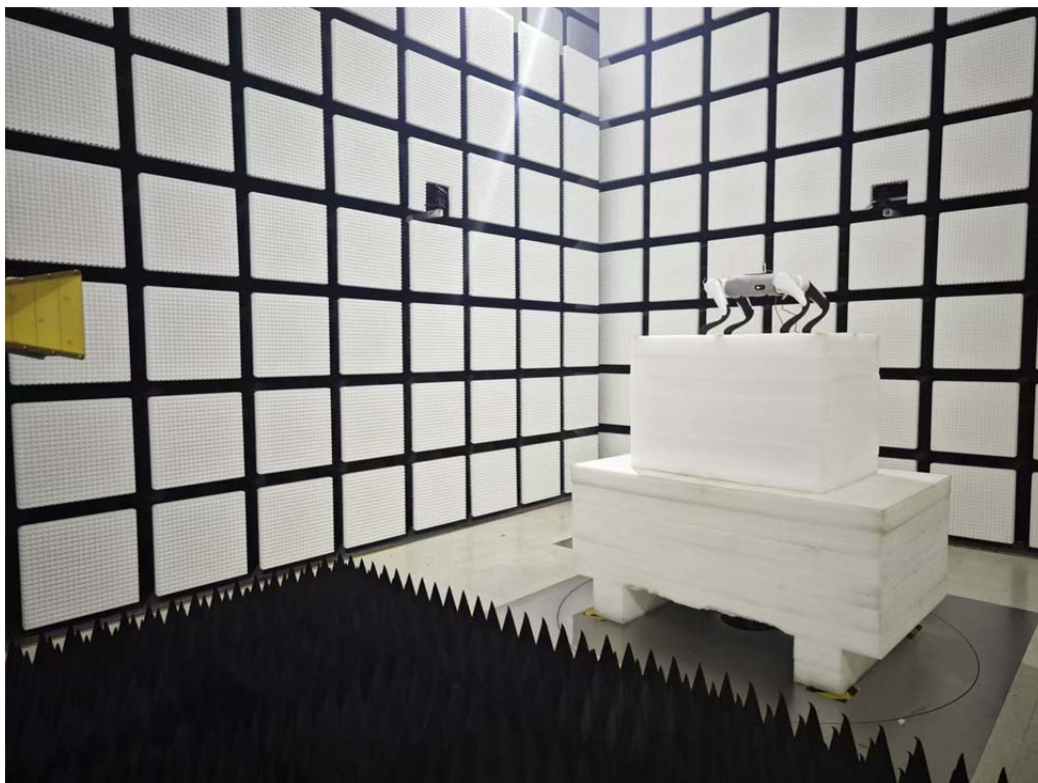
Radiated Emission Above 1-18GHz View
