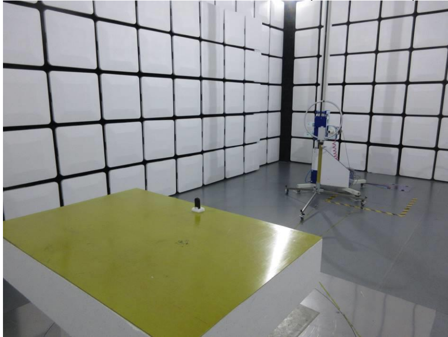
RADIATED RF MEASUREMENT SETUP (9kHz ~ 30 MHz)
