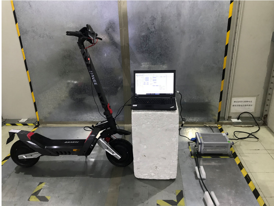
Conducted Emissions (Left View)
