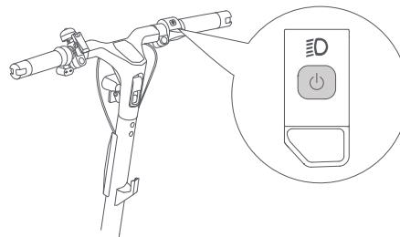
Press the button to turn the scooter on, and hold the button for 2 to 3 seconds to turn the scooter off. When the scooter is on, press twice to change riding modes.
