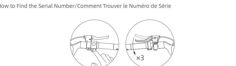
EN Press the accelerator and squeeze the brake lever 3 times to activate the scooter's serial number search function. The serial number will then be displayed in the Find My app (for iOS users who have paired the scooter using the Find My app).
