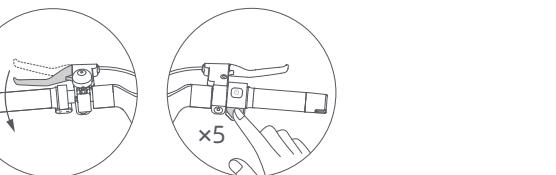
EN Turn the scooter on. Make sure the scooter is not locked or during charging, squeeze the brake lever and simultaneously press the accelerator 5 times, when the display is off, the scooter has been restored to factory settings, and the scooter cannot be searched for by the Find My app. If you need to pair again, delete the added scooter from the Find My app and then pair it again.
