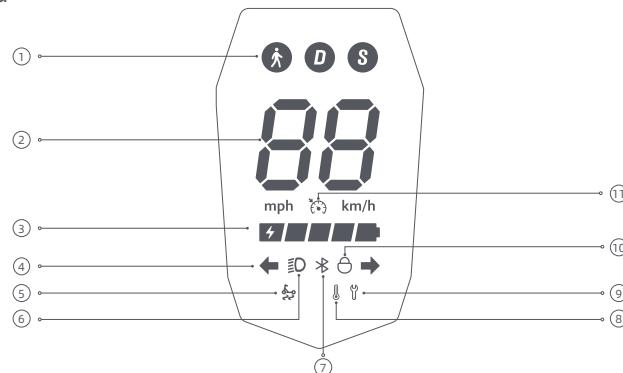
① Riding Modes: is for walking mode, and its maximum speed is 6 km/h. is for standard mode. is for sport mode.
