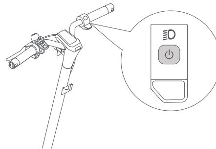
Press the button to turn the scooter on, and hold the button for 2 to 3 seconds to turn the scooter off. When the scooter is on, press twice to change riding modes.
