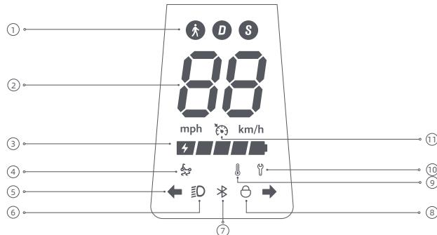
① Riding Modes: is for walking mode, and its maximum speed is 6 km/h. D is for standard mode. S is for sport mode.
