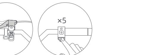
EN Turn the scooter on. Make sure the scooter is not locked or during charging, squeeze the brake lever and simultaneously press the accelerator 5 times, when the display is off, the scooter has been restored to factory settings, and the scooter cannot be searched for by the Find My app. If you need to pair again, delete the added scooter from the Find My app and then pair it again.
